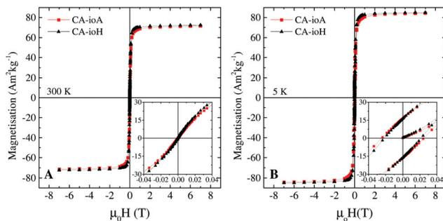
**Fig. 2** Representative  $M(H)$  magnetisation curves of samples CA-ioA and CA-ioH at (A) 300 K and (B) 5 K, showing the transition from a room temperature superparamagnetic state to a low temperature blocked state.
