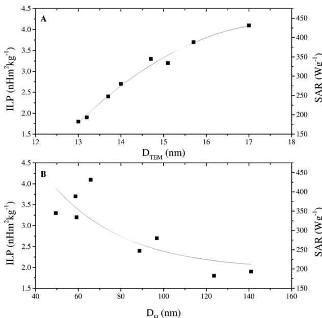
**Fig. 3** (A) ILP versus core size  $D_{TEM}$  and (B) ILP versus hydrodynamic diameter  $D_H$  for the citric acid coated iron oxide nanoparticle series listed in Table 1. SAR values are also indicated for reference. Solid lines are a guide to the eye.
