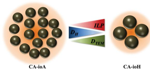
**Scheme 1** Schematic of the observed correlation between the intrinsic loss parameter ILP, hydrodynamic diameter  $D_H$ , and core particle diameter  $D_{TEM}$ , for the citric acid coated multi-core iron oxide nanoparticles in this study. The increase in core size, together with the decrease in the hydrodynamic size, leads to a decrease of the number of cores per multi-core system ( $N$ ), a decrease in the demagnetising interactions between those cores, and an increase in the ILP.
