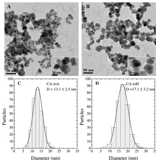
**Fig. 1** TEM analysis of samples (A) CA-ioA and (B) CA-ioH. Core size distributions were obtained from the measurement of at least 300 cores per sample for (C) CA-ioA and (D) CA-ioH. Size distributions were fitted with a normal function (solid line).
