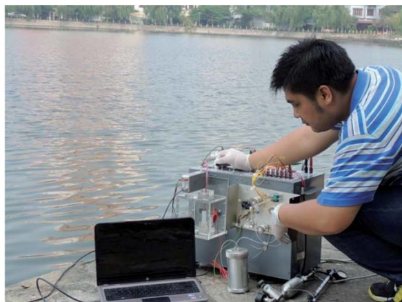
Fig. 1 (A) A block-diagram demonstrating the basic set-up of a CE system with some optional automatable parts; (B) demonstration of an in-house-made CE system in operation. Pt: platinum electrode; W: waste; GND: ground electrode; BGE: background electrolyte; HV: high voltage; C 4 D: capacitively coupled contactless conductivity detector.
