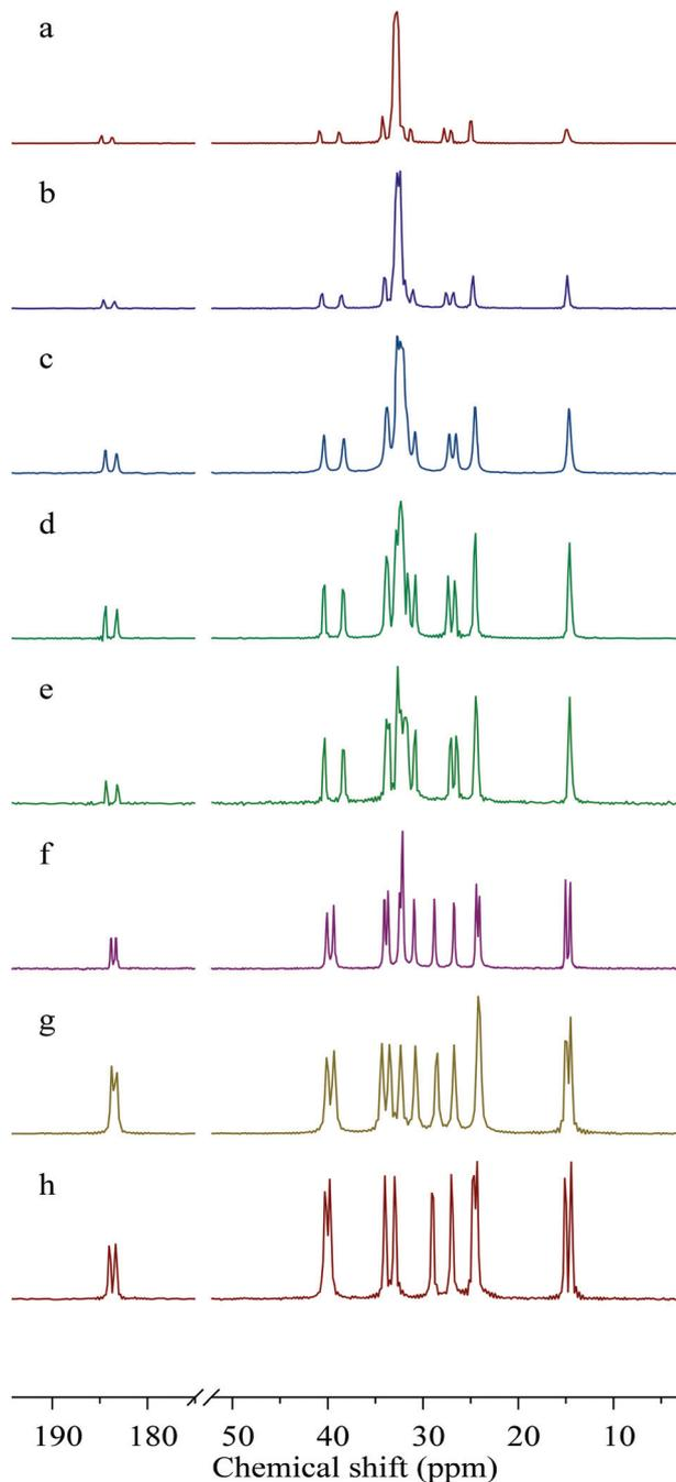
**Fig. 1**  $^{13}\text{C}$  NMR spectra of lead carboxylates obtained with cross polarization and proton decoupling spinning at 12 kHz. (a) Lead octadecanoate, (b) lead hexadecanoate, (c) lead undecanoate, (d) lead decanoate, (e) lead nonanoate, (f) lead octanoate, (g) lead heptanoate, and (h) lead hexanoate. The spectra show that the lead carboxylates can be divided into two subgroups, shorter chains (C6–C8) having a larger span than the long-chain carboxylates (C9–C11, C16, and C18).
