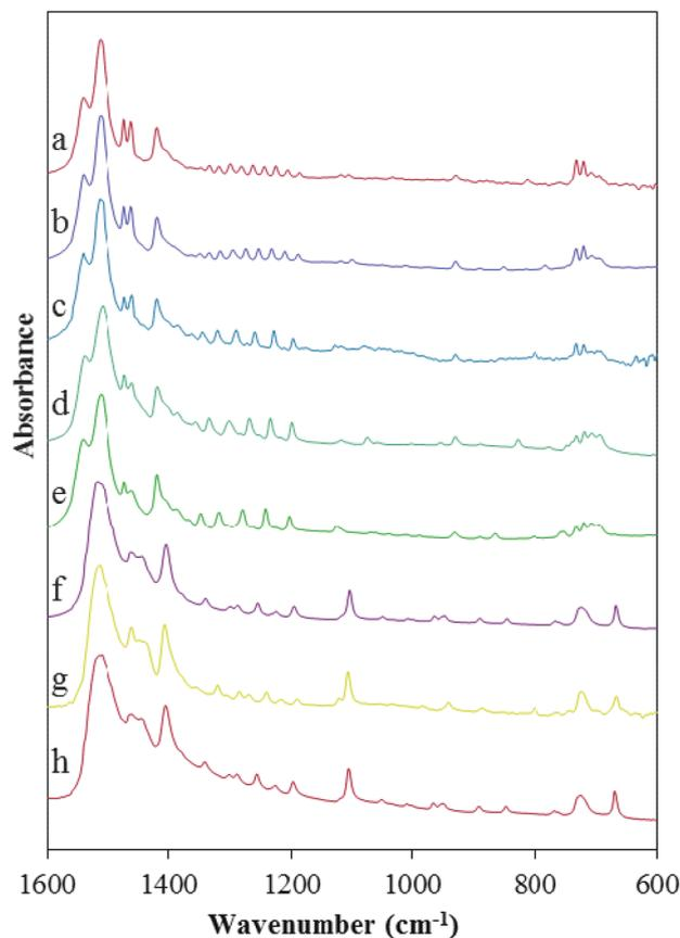
**Fig. 3** FTIR spectra of (a) lead octadecanoate, (b) lead hexadecanoate, (c) lead undecanoate, (d) lead decanoate, (e) lead nonanoate, (f) lead octanoate, (g) lead heptanoate, and (h) lead hexanoate. The FTIR spectra show differences in the two subgroups (short- and long-chain lead carboxylates) in the ranges 1515–1540  $\text{cm}^{-1}$ , 1150–1350  $\text{cm}^{-1}$ , and around 720  $\text{cm}^{-1}$ .
