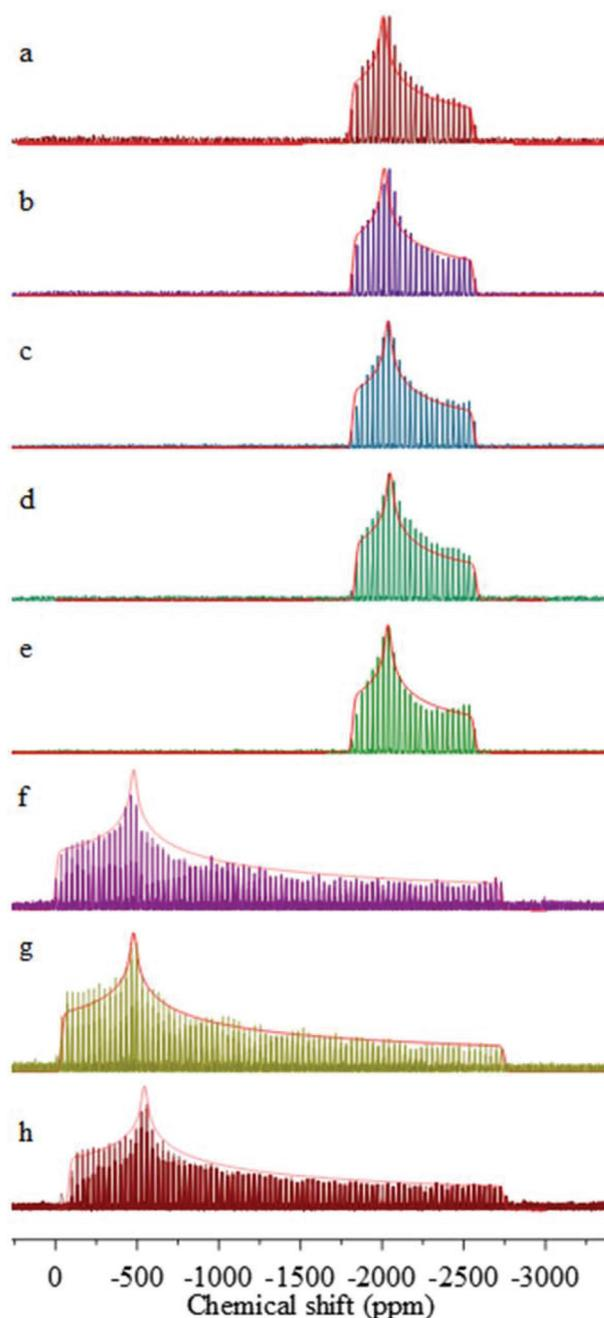
**Fig. 2**  $^{207}\text{Pb}$  NMR spectra of lead carboxylates obtained with WURST-CPMG. (a) Lead octadecanoate, (b) lead hexadecanoate, (c) lead undecanoate, (d) lead decanoate, (e) lead nonanoate, (f) lead octanoate, (g) lead heptanoate, and (h) lead hexanoate. The spectra show that the lead carboxylates can be divided into two subgroups, shorter chains (C6–C8) having a larger span than the long-chain carboxylates (C9–C11, C16, and C18).
