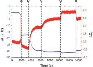
Fig. 3 Plot of frequency and dissipation change over time, calculated from the frequency values of the seventh overtone. Marked timepoints indicate when each component reached the sensor: (a) Bt-DOPC vesicles – 'burst effect', (b) avidin, (c) Bt-APTES-MNPs, (d) biotin, (e) 'blank' buffer.
