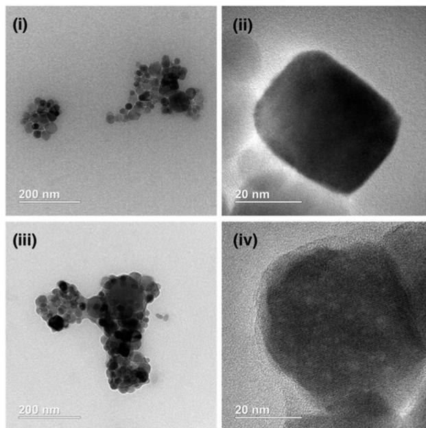
Fig. 2 Representative HRTEM images of (i) and (iii) uncoated Fe<sub>3</sub>O<sub>4</sub> MNPs and (ii) and (iv) APTES coated commercial Fe<sub>3</sub>O<sub>4</sub> MNPs.
