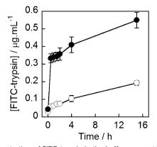
Fig. 6 Concentration of FITC-trypsin in the buffer supernatant of MNPV samples ( $\bigcirc$ ) not exposed to AMF, ( $\bigcirc$ ) AMF exposed. AMF pulse completed at t=5 minutes.
