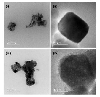
Fig. 2 Representative HRTEM images of ((i) and (ii)) uncoated  $Fe_3O_4$  MNPs and ((iii) and (iv)) APTES coated commercial  $Fe_3O_4$  MNPs.
