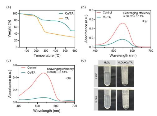
Fig. 5 (a) TGA curves of TA and Cu/TA nanozyme. (b) Absorption spectra of solutions after reaction with  ${}^{\bullet}O_2^{-}$ . (c) Absorption spectra of solutions after reaction with  ${}^{\bullet}O_1$ . (d) Photographs of  $H_2O_2$  decomposing to produce  $O_2$  in 5 min in the absence and presence of Cu/TA nanozyme.
