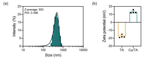
(a) Hydrodynamic particle size distribution and (b) zeta potential of Cu/TA nanozyme.
