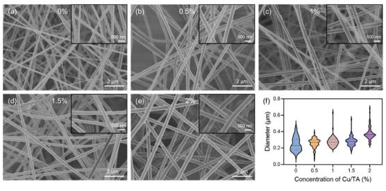
Fig. 8 (a-e) SEM images and (f) fiber diameter distribution of CTP membranes at various Cu/TA nanozyme concentrations.
