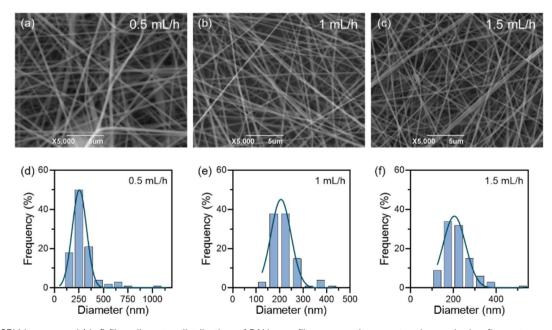
Fig. 7 (a-c) SEM images and (d-f) fiber diameter distribution of PAN nanofibrous membranes at various spinning flow rates
