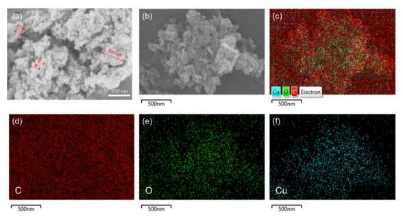
Fig. 3 (a) SEM image and (b-f) EDS elemental analysis of Cu/TA nanozyme.
