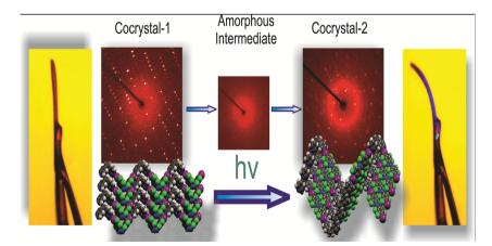
Fig. 6 Photoinduced bending of halogen-bonded cocrystals followed by in situ X-ray diffraction reveals that the transition from the unbent cis single crystal to the bent polycrystalline trans state proceeds through an amorphous intermediate phase. Reproduced with permission from ref. 100. Copyright 2014, The Royal Society of Chemistry.
