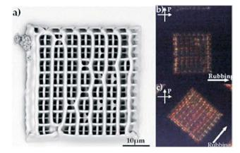
Fig. 5 Left: a 4-layer woodpile structure with 5 μm line distance and 1.3 µm distance between two consecutive layers. The structure is obtained by direct laser writing of azobenzene-containing LC elastomers. Right: polarized-optical micrographs of the LC elastomer woodpiles at different angles of the LC alignment direction with respect to the analyzer. Reproduced with permission from ref. 86. Copyright 2014, Wiley-VCH.
