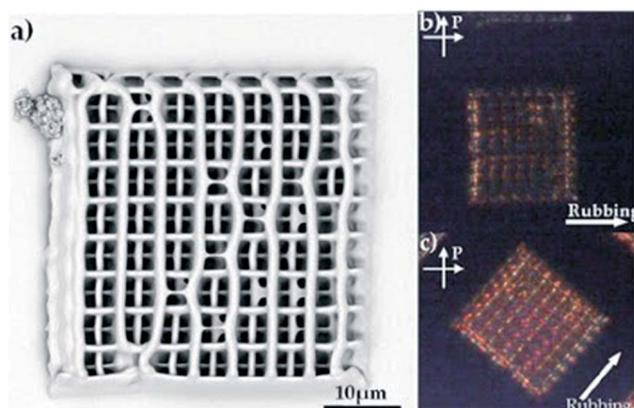
Fig. 5 Left: a 4-layer woodpile structure with 5  $\mu\text{m}$  line distance and 1.3  $\mu\text{m}$  distance between two consecutive layers. The structure is obtained by direct laser writing of azobenzene-containing LC elastomers. Right: polarized-optical micrographs of the LC elastomer woodpile at different angles of the LC alignment direction with respect to the analyzer. Reproduced with permission from ref. 86. Copyright 2014, Wiley-VCH.
