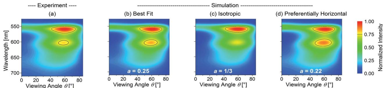
Fig. 2 TM-polarized part of the spectral radiant intensity for the OLED stack with  $\text{Ir}(\text{dhfp})_2(\text{acac})$ . (a) Experimental data, (b) simulated data for the best fit ( $a = 0.25$ ), (c) simulation assuming isotropic orientation ( $a = 1/3$ ) and (d) simulation assuming slightly stronger horizontal orientation ( $a = 0.22$ ). All intensities are normalized to the maximum intensity and are plotted on a linear false-color scale.
