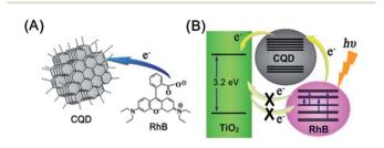
Fig. 25 (A) Scheme of electron transfer from RhB to CQDs. (B) CQDs serve as an electron transfer intermediary for bridging the photogenerated electrons and suppressing their recombination. Adapted with permission. 117 Copyright 2013, American Chemical Society.
