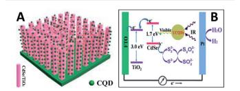
Fig. 29 (A) A schematic diagram showing the CQD/CdSe/ $TiO_2$  NR photoanode. (B) A schematic diagram to illustrate how up-conversion of the carbon quantum dots (UCQDs) served as spectral converters for the CdSe/ $TiO_2$  NR photoanode. Adapted with permission. <sup>126</sup> Copyright 2013, Royal Society of Chemistry.
