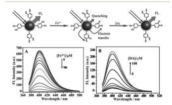
Fig. 30 (Up) Schematic representation of fluorescent CQDs for the detection of Fe<sup>3+</sup> ions and dopamine. (A) Representative fluorescence emission spectra of CQDs in the presence of increasing Fe<sup>3+</sup> concentration (0-700 μM) in a HEPES buffer (10 mM) at pH 7.0. (B) Fluorescence emission spectra of CQDs containing Fe $^{3+}$  (600  $\mu$ M) with increase in DA concentration (0-100 μM). Adapted with permission. 61 Copyright 2013, Wiley-VCH.
