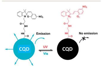
Fig. 8 Schematic illustration of the light-induced fluorescence modulation of spiropyran-functionalized CQDs. Adapted with permission.<sup>59</sup> Copyright 2013, Royal Society of Chemistry.
