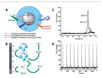
Fig. 15 (A) Schematic illustration of the PL and ECL emissions of CQDs. (B) The mechanism of ECL in the o-CQDs/ $K_2S_2O_8$  system. (C) ECL profiles of o-CQDs at a scan rate of 0.01 and 0.05 V s<sup>-1</sup>. (D) The reproducibility of ECL in a continuous scan mode. Adapted with permission. Recopyright 2013, Wiley-VCH.
