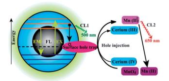
Fig. 14 Schematic illustration of the FL and CL mechanisms in the CQDs-KMnO<sub>4</sub> and CQDs-cerium(IV) systems. CL1 and CL2 represent two CL routes in the system. Adapted with permission.<sup>73</sup> Copyright 2012, Royal Society of Chemistry.
