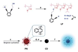
Fig. 7 Preparation of soluble CQDs with tunable sizes from singlechain polymeric nanoparticles. Adapted with permission.8 Copyright 2013, Royal Society of Chemistry.
