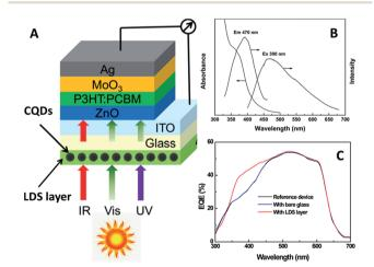
Fig. 26 (A) Schematic architecture of the BHJ solar cell with LDS layer. (B) UV-vis absorption and PL spectra of the CQDs filled polysiloxane composite (~20 μm thick) coated on glass. (C) Wavelength dependences of external quantum efficiency of the P3HT:PCBM-based solar cell with and without the LDS layer. Adapted with permission.<sup>71</sup> Copyright 2014, Elsevier.
