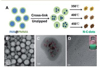
Fig. 6 Scheme of preparing CQDs from polymeric nanoparticles (A) and the TEM images of the core-shell polymeric nanoparticles (B), core cross-linked polymeric nanoparticles (C) and final CQDs (D). The digital image of the CQDs solution is shown in the inset. Adapted with permission.<sup>42</sup> Copyright 2013, Royal Society of Chemistry.
