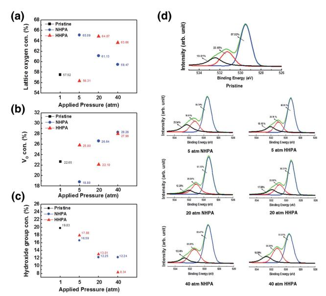
Fig. 1 Compositions of NiO<sub>x</sub> by O 1s XPS spectra divided into (a) lattice oxygen, (b)  $V_O$ , and (c) loosely bound hydroxide related group concentrations. (d) The overall bulk XPS spectra of pristine, NHPA (5, 20, and 40 atm), and HHPA (5, 20, and 40 atm) NiO<sub>x</sub> thin films.
