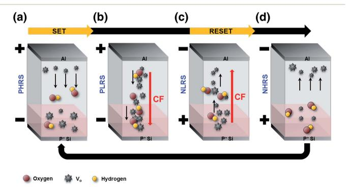
Fig. 6 Schematic of the operation of the HHPA treated device. The enhanced concentrations of  $V_{\rm O}$  at the interface and bulk layer result in the improved device distribution and high LRS/HRS possible.
