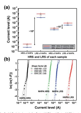
**Fig. 3** (a) Statistical graph for 5 atm HHPA and 5 atm NHPA treated devices. 30 sequential sweepings were measured for the HRS and LRS parameters. (b) The Weibull distributions for 5 atm HHPA and NHPA devices. The HHPA device shows a quite large LRS/HRS ratio while the NHPA treated device demonstrates a small ratio with better distribution.
