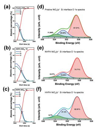
Fig. 5 Composition profiles for (a) pristine, (b) NHPA, and (c) HHPA treated devices. The cross-sectional O 1s spectra were recorded at the bottom interfaces (contents of Ni  $\stackrel{.}{=}$  Si) of (d) pristine, (e) NHPA, and (f) HHPA treated devices.
