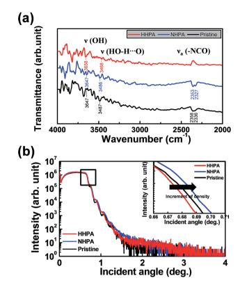
Fig. 4 (a) FT-IR spectra to observe the chemical parameter variations in 5 atm HHPA, 5 atm NHPA, and pristine  $NiO_{x}$ . (b) XRR spectra were also recorded to check the variations in physical parameters in 5 atm HHPA, 5 atm NHPA, and pristine  $NiO_{x}$ .
