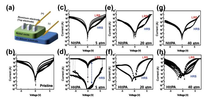
Fig. 2 (a) Demonstrated  $Al/sol-NiO_x/Si$  structure and I-V characteristics from the initial to the 5<sup>th</sup> cycle for (b) pristine, (c) 5 atm NHPA, (d) 5 atm HHPA, (e) 20 atm NHPA, (f) 20 atm HHPA, (q) 40 atm NHPA, and (h) 40 atm HHPA treated  $NiO_x$  based devices.
