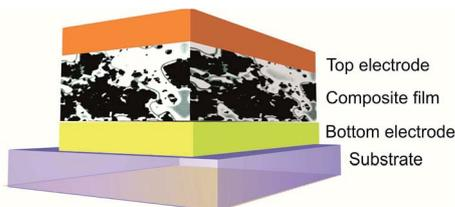
Fig. 1 Schematic structure of a memory device.
