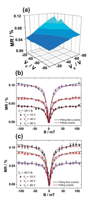
Fig. 6 (a) A "landscape" of MR values measured at different  $V_d$  and  $V_g$ for bilayer thin films of F6-TNAP (5 nm)/Spiro-TAD (40 nm) field-effect transistor fabricated on bare SiO2. Magnetic field dependence of MR measured at (b) constant  $V_{\rm d}$  for different  $V_{\rm g}$  and at (c) constant  $V_{\rm g}$  for different  $V_d$ . The corresponding data were plotted by using non empirical laws of non-Lorentzian and Lorentzian line shapes.
