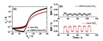
Fig. 3 (a) Transfer characteristics of bilayer F6-TNAP (5 nm)/Spiro-TAD (40 nm) field-effect transistors fabricated on bare SiO<sub>2</sub> and HMDS-treated  $SiO_2$  measured at  $V_d = -30$  V. (b) MR effect of both devices recorded at  $V_{\rm d} = V_{\rm g} = -30$  V.
