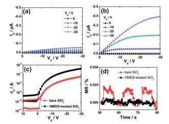
Fig. 2 Output curves of Spiro-TAD field-effect transistors fabricated on (a) bare SiO<sub>2</sub> and (b) HMDS-treated SiO<sub>2</sub>. (c) The corresponding transfer curves were recorded at  $V_{\rm d} = -30$  V. (d) The MR effects of both devices were measured at  $V_{\rm d} = V_{\rm g} = -40$  V (for bare  ${\rm SiO_2}$ ) and  $V_{\rm d} = V_{\rm g} = -50 \text{ V}$  (for HMDS-treated SiO<sub>2</sub>).
