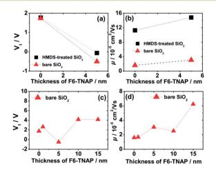
Fig. 4 (a) The fitted threshold voltage  $V_t$  and (b) hole mobility  $\mu$  of F6-TNAP/Spiro-TAD field-effect transistors fabricated on bare SiO<sub>2</sub> and HMDS-treated SiO<sub>2</sub>. (c)  $V_t$  and (d)  $\mu$  of F6-TNAP/Spiro-TAD devices fabricated on bare SiO<sub>2</sub> with different thicknesses of F6-TNAP.
