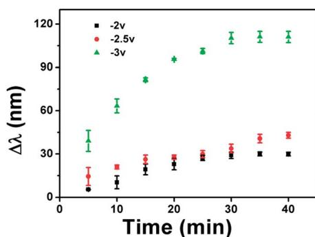
Fig. 4 Change in the reflectance peak position ( $\Delta\lambda$ ) as a function of time for various applied potentials. Here,  $\Delta\lambda$  is  $\lambda_t - \lambda_{\text{original}}$ , where  $\lambda_t$  is the position of the peak at a given time after applying a given potential and  $\lambda_{\text{original}}$  is the initial position of the peak. Each data point is the average of 3 experiments, with the error bars as the standard deviation.
