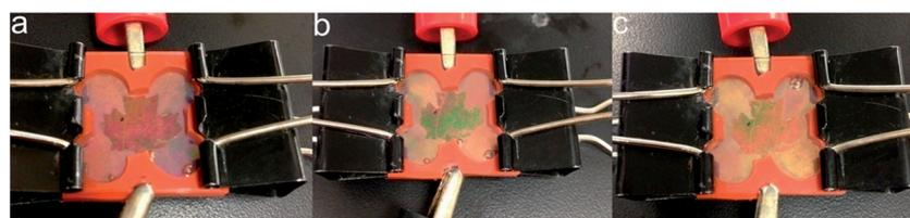
Fig. 6 Photographs of a patterned etalon in an electrochemical cell at: (a) 0 V, (b) 2 V, and (c) -2 V.
