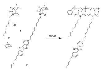
Scheme 3 Polymerisation of norbornene-BTBT with either norbornene or alkyl norbornene imide.
