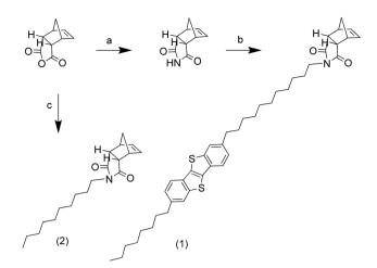
Scheme 2 Synthesis of molecules 1 and 2. (a) 1 eq. NH<sub>4</sub>OAc, AcOH, 140 °C, 16 h, 100%. (b) 1 eq. C<sub>8</sub>BTBTC<sub>11</sub>Br (0.5 g), 1.5 eq. K<sub>2</sub>CO<sub>3</sub>, 1:1 DMF: THF, reflux, 16 h, 96%. (c) 1 eq. 1-decylamine, 1 eq. triethylamine, Ar, dry toluene, reflux, 16 h, Dean-Stark app., 86%
