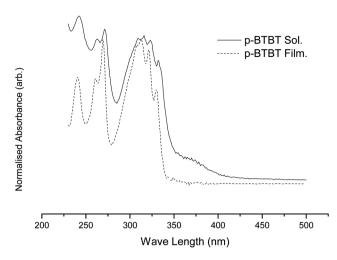
Fig. 3 Typical UV-vis of ROMP polymers in solution and thin film.
