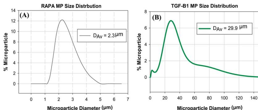
Fig. 1 Microparticle size determined using dynamic light scattering techniques for (A) Phagocytosable MPs (average diameter  $\sim 2.3 \mu\text{m}$ ) and, (B) Un-phagocytosable (average diameter  $\sim 30 \mu\text{m}$ ).
