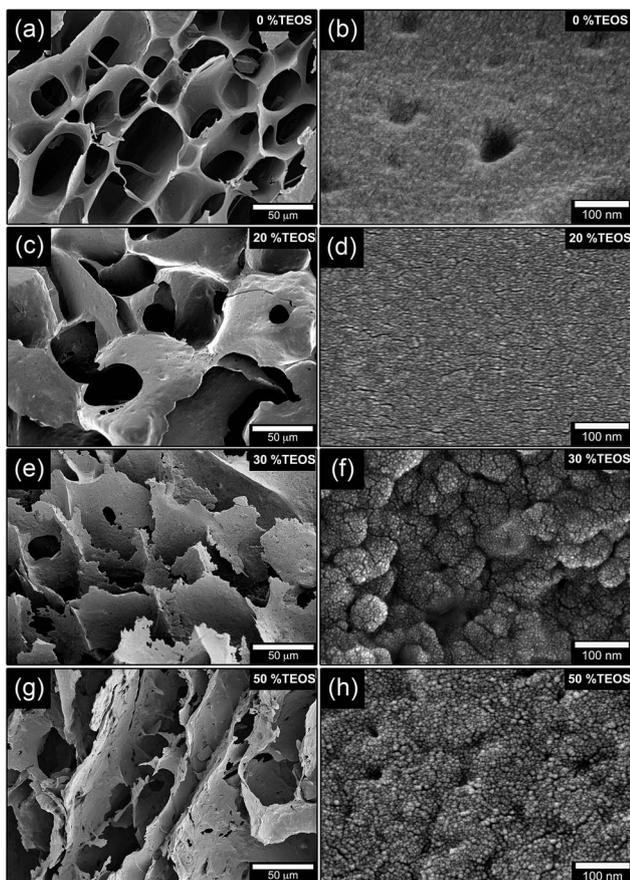
Fig. 3 FE-SEM images of foams frozen at  $-25\text{ }^{\circ}\text{C}$  prepared with (a) 0, (c) 20, (e) 30 and (g) 50% TEOS. Images (b), (d), (f), and (h) correspond to magnified areas of, respectively, the 0, 20, 30 and 50% TEOS foams.
