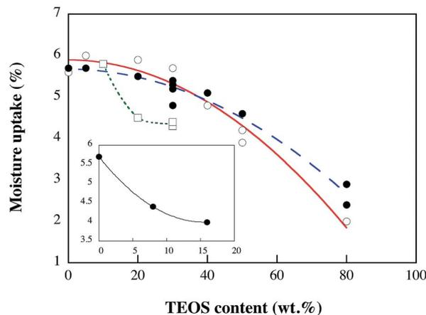
Fig. 9 Moisture content as a function of silica (TEOS) content; foams prepared at  $-25\text{ }^\circ\text{C}$  ( $\circ$ ), at  $-196\text{ }^\circ\text{C}$  ( $\bullet$ ), cross-linked with 8% GA ( $\square$ ) and 16% GA (inset curve). The overall standard deviation was  $\pm 9\%$  of the value, as estimated from 60 measurements on WG and silica-WG foams.
