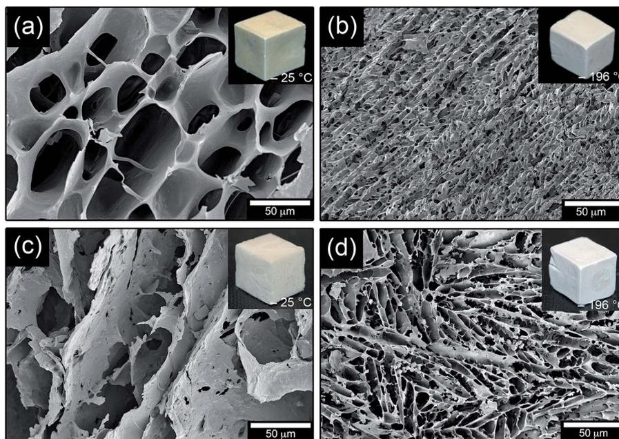
Fig. 4 FE-SEM images of foams frozen at  $-25\text{ }^{\circ}\text{C}$  prepared with (a) 0 and (c) 50% TEOS. Foams frozen at  $-196\text{ }^{\circ}\text{C}$  prepared with 0 and 50% TEOS are shown in (b) and (d).
