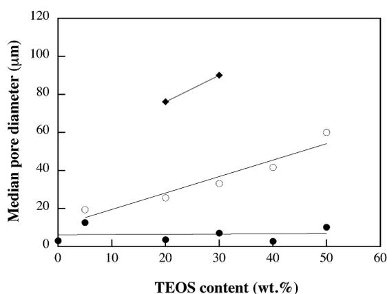
Fig. 5 Median pore diameter as a function of TEOS content; foams frozen at  $-25\text{ }^{\circ}\text{C}$  without (○) and with (◆) crosslinker (8% glutaraldehyde). Also shown are foams frozen at  $-196\text{ }^{\circ}\text{C}$  (●).
