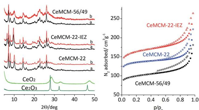
Fig. 1 XRD for  $\text{CeO}_2$ ,  $\text{Ce}_2\text{O}_3$  and Ce-MCM-22, Ce-MCM-22-IEZ, and Ce-MCM-56/49 zeolites, (a) calcined and cerium-exchanged, (b) cerium-exchanged and vacuum activated samples;  $\text{N}_2$  isotherms for calcined samples.
