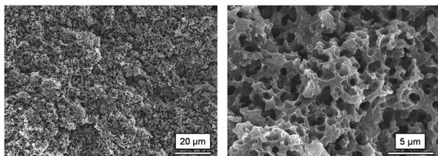
Fig. 3 SEM micrographs of the CDC monoliths.
