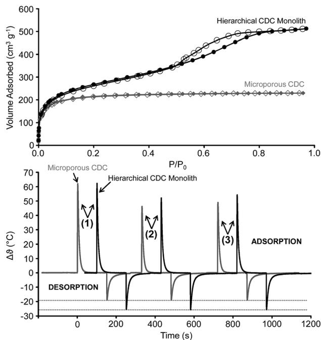
Fig. 4 Top: Volumetric *n*-butane adsorption/desorption (filled symbols/empty symbols) isotherms of the hierarchical CDC-Ms and a purely microporous CDC (diamonds) measured at 5 °C ( $P_0 \sim 1.25 \text{ bar}$ ). Bottom: thermal response measurements of *n*-butane adsorption (1 bar, 25 °C) in activated (1) hierarchical CDC-Ms (black, horizontally shifted by 100 s) and a purely microporous CDC (grey) and after desorption times of 120 s (2) and 150 s (3).
