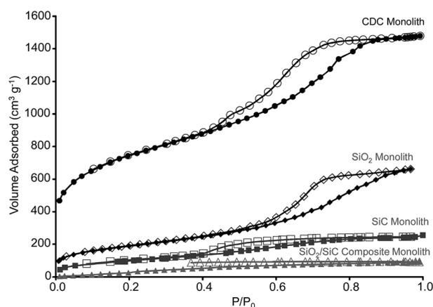
Fig. 1 Nitrogen adsorption/desorption (filled symbols/empty symbols) isotherms of the CDC monoliths (circles), SiO<sub>2</sub> monoliths (diamonds), SiC monoliths (squares), and SiO<sub>2</sub>/SiC composite monoliths (triangles) measured at -196 °C.
