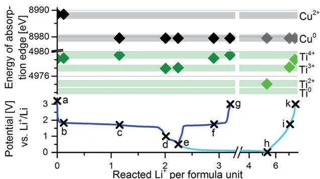
Fig. 6 Change of the energy of the copper- and the titanium absorption edge at half of the edge step of *ex situ* samples of  $\text{Cu}_{0.5}\text{TiOPO}_4$ . The position of the absorption edge of the measured reference materials is shown as well. At the bottom, the corresponding galvanostatic curve is plotted.
