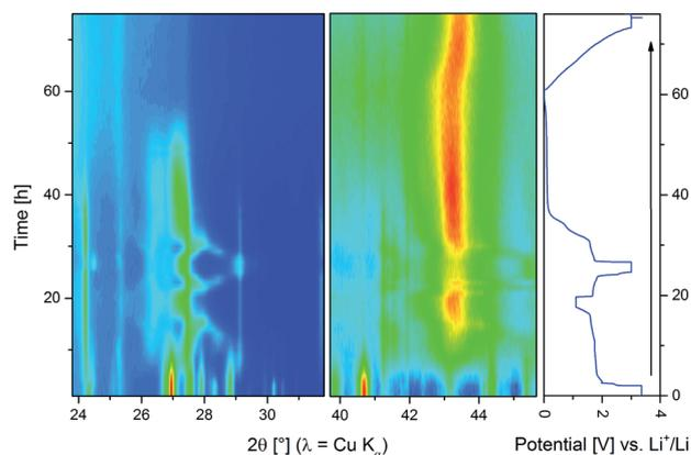
Fig. 2 Contour plot of an *in situ* XRD measurement at a specific current of  $16.9 \text{ A kg}^{-1}$  (blue: low intensity; red: high intensity). On the right hand side, the corresponding galvanostatic curve is shown.
