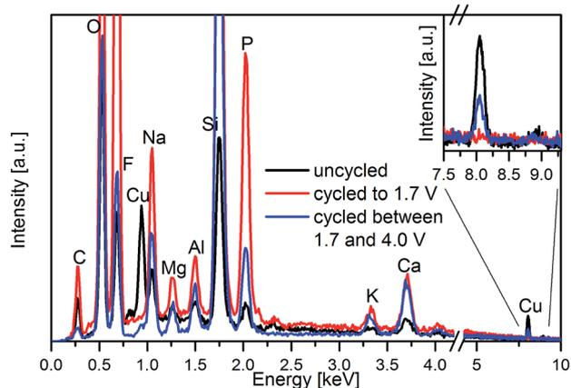
Fig. 9 EDX spectra of lithium counter electrodes and working electrodes of  $\text{Cu}_{0.5}\text{TiOPO}_4$  after cycling to 1.7 V, cycling 10 times between 1.7 V and 4.0 V, and an uncycled cell (all stored for two weeks after assembly).
