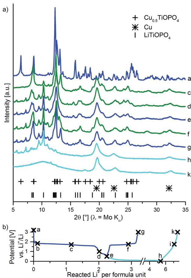
Fig. 3 (a) *Ex situ* XRD measurements of  $\text{Cu}_{0.5}\text{TiOPO}_4$  cycled to key points in the first cycle. (b) shows the corresponding galvanostatic curve.
