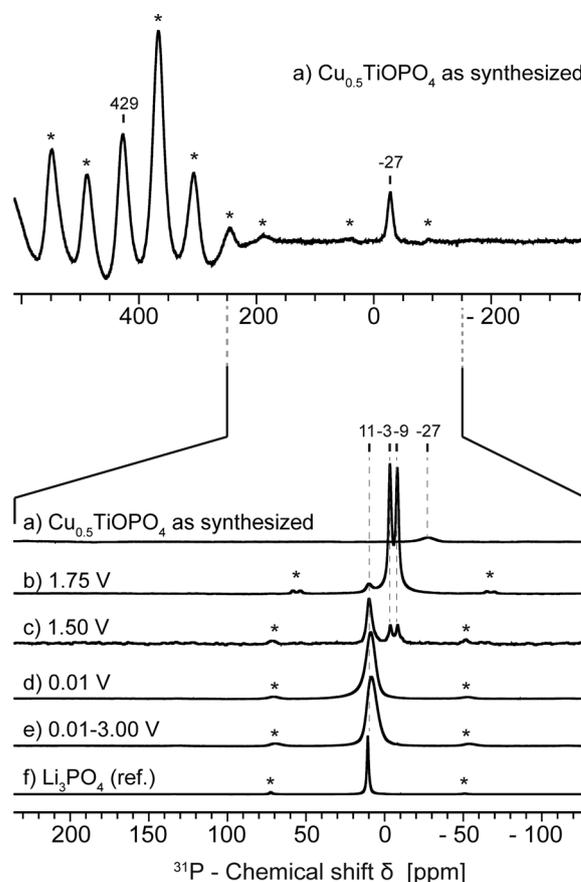
Fig. 7  $^{31}\text{P}$  MAS NMR spectra of *ex situ* samples of  $\text{Cu}_{0.5}\text{TiOPO}_4$  and pure  $\text{Li}_3\text{PO}_4$ . The top spectrum is an addition of two spectra acquired at two different transmitter positions (0 ppm and 250 ppm) to cover a larger window width. For all the spectra the number of scans was 512 K and the recycling delay was set to 1 s.
