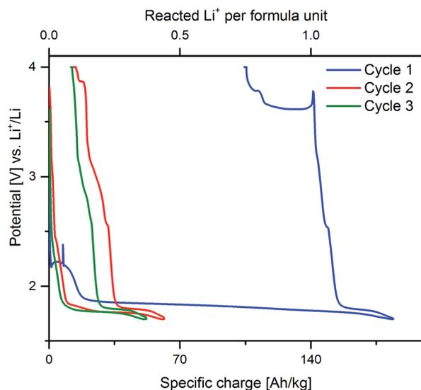
Fig. 8 Galvanostatic curve of  $\text{Cu}_{0.5}\text{TiOPO}_4$  cycled 3 times between 1.7 V and 4.0 V with a specific current of  $14.06 \text{ A kg}^{-1}$ .
