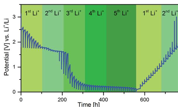
Fig. 1 GITT-measurement during the first cycle of  $\text{Cu}_{0.5}\text{TiOPO}_4$ .
