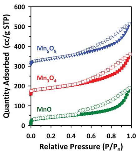
Fig. 6 Nitrogen adsorption–desorption isotherms of converted manganese oxides.
