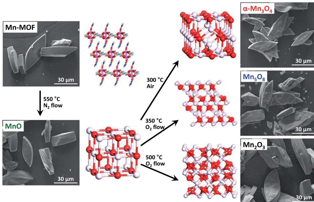
Fig. 1 SEM images and atomic structures of Mn-MOF and converted manganese oxides during structural transformation of Mn-MOF into MnO, Mn<sub>3</sub>O<sub>4</sub>, Mn<sub>5</sub>O<sub>8</sub> and Mn<sub>2</sub>O<sub>3</sub>.
