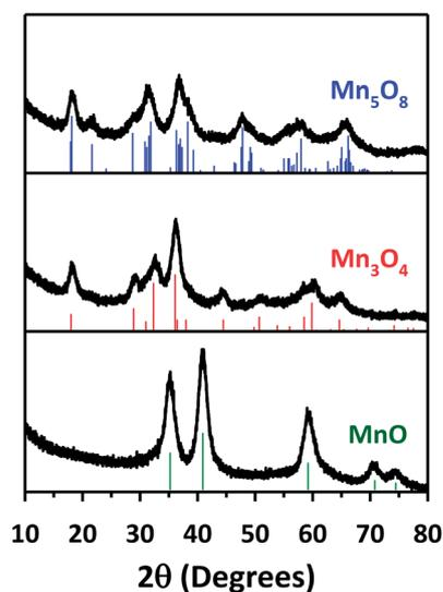
Fig. 4 XRPD patterns of converted manganese oxides.
