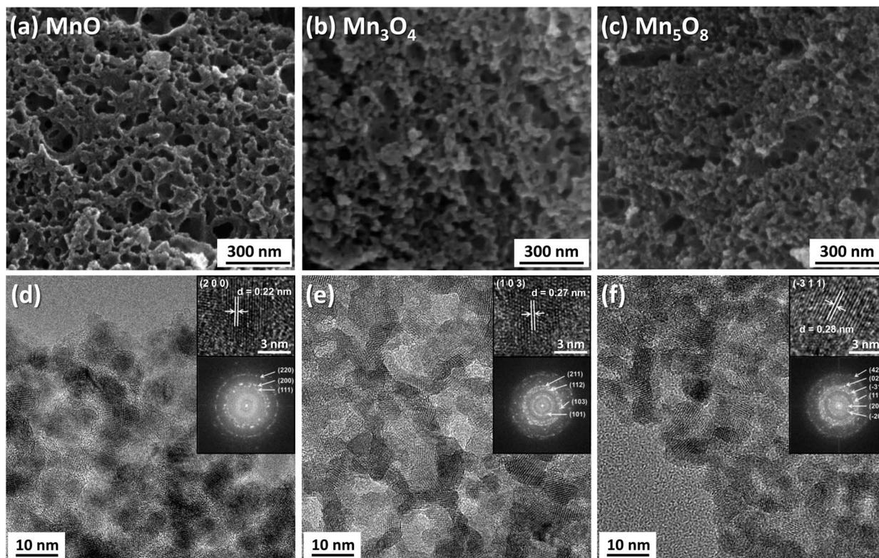
Fig. 3 Characterization of converted manganese oxides. (a–c) SEM images, (d–f) TEM images, and (d–f, insets) HR-TEM images and electron diffraction patterns of nanoporous MnO (a and d),  $\text{Mn}_3\text{O}_4$  (b and e), and  $\text{Mn}_5\text{O}_8$  (c and f).
