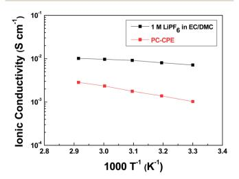
Fig. 4 Temperature-dependent ionic conductivity (temperature range  $=30-70\,^{\circ}\text{C})$  of PC-CPE and carbonate-based liquid electrolyte (1 M LiPF $_{6}$  in EC/DMC  $=1/1\,\text{v/v}).$
