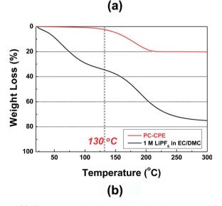
Fig. 7 (a) Photographs showing the swelling behavior of cells assembled with PC-CPE or carbonate-based liquid electrolyte (1 M LiPF<sub>6</sub> in EC/DMC = 1/1 v/v), after exposure to thermal shock (=130 °C/0.5 h). (b) Dynamic mode TGA profiles of PC-CPE and carbonate-based electrolyte (1 M LiPF<sub>6</sub> in EC/DMC = 1/1 v/v).
