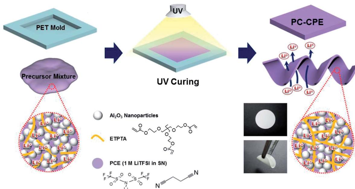
**Scheme 1** A schematic representation of the UV curing-assisted fabrication process for PC-CPE, wherein chemical structures and photographs depicting mechanical bendability of PC-CPE are also provided.
