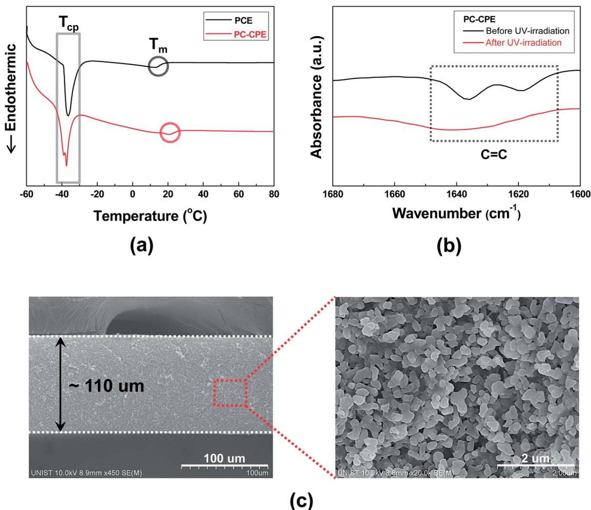
Fig. 1 Structural characterization of PC-CPE: (a) DSC profiles showing characteristic transition temperatures ( $T_{CP}$  and  $T_m$ ) of SN in PCE and PC-CPE; (b) FT-IR spectra (before/after UV curing) of acrylic C=C bonds of ETPTA in PC-CPE; (c) cross-sectional FE-SEM images of PC-CPE, wherein the high-magnification view exhibits the presence of well-reticulated interstitial voids (originally occupied with PCE) formed between the  $\text{Al}_2\text{O}_3$  nanoparticles.
