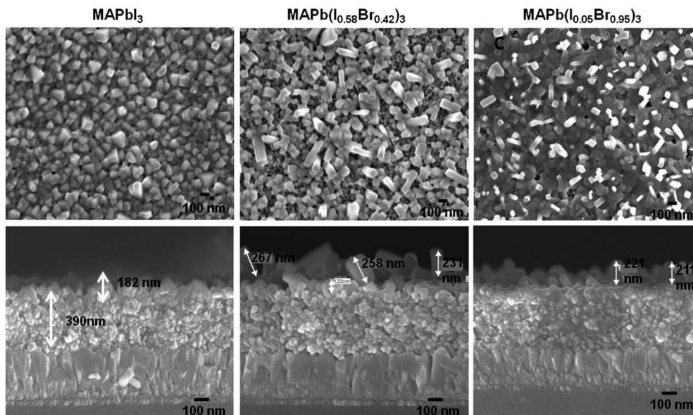
Fig. 4 Field emission microscopic (FESEM) images of mixed halide perovskite films with different halides namely;  $\text{MAPbI}_3$ ,  $\text{MAPb}(\text{I}_{0.58}\text{Br}_{0.42})_3$  and  $\text{MAPb}(\text{I}_{0.05}\text{Br}_{0.95})_3$ ; top (first row) and cross-sectional view (second row).
