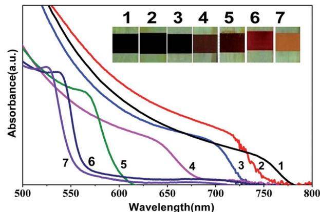
Fig. 1 UV-Vis absorption spectra of the mixed halide lead perovskite ( $\text{MAPb}(\text{I}_{1-x}\text{Br}_x)_3$  ( $0 \leq x \leq 1$ )) films formed *via* a sequential deposition process. The numbers 1–7 correspond to the mixed lead halide perovskite films with different halide (iodide/bromide) compositions as estimated in the corresponding table. The inset shows the photographs of mixed lead halide nanocomposite perovskite films on FTO substrates.
