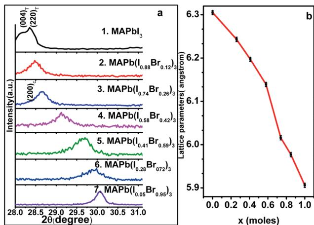
Fig. 2 Powder X-ray diffraction analysis of mixed lead halide perovskite films  $\text{MAPb}(\text{I}_{1-x}\text{Br}_x)_3$  ( $0 \leq x \leq 1$ ) in the region of the tetragonal (004)T & (220)T and cubic (200)C reflections ( $2\theta = 27.5\text{--}31.0^\circ$ ); (b) lattice parameters of pseudocubic or cubic  $\text{MAPb}(\text{I}_{1-x}\text{Br}_x)_3$  as a function of the Br content ( $x$ ) in moles along with the precision of experimental data fitting.
