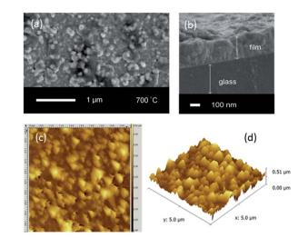
Fig. 2 (a) A typical top-down SEM image (b) side-on SEM image, (c) a  $5 \mu m$  field size AFM image and (d) the corresponding 3D AFM image of the BiFeO<sub>3</sub> film formed after annealing at 700 °C.
