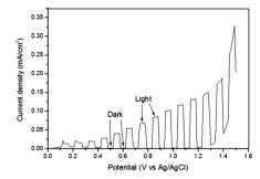
Fig. 4 I-V curve for a BiFeO<sub>3</sub> film deposited on FTO glass via AACVD.
