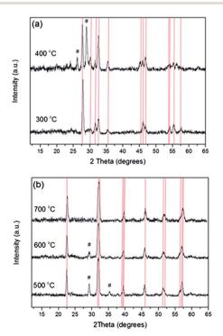
Fig. 1 (a) X-ray diffraction patterns of BFO films annealed at 300 °C (as-deposited) and 400 °C. Red lines correspond to  $Bi_{24}Fe_2O_{39}$  (PDF = 042-0201). (b) X-ray diffraction patterns of films annealed at temperatures between 500 and 700 °C. Red lines correspond to BiFeO<sub>3</sub> (PDF = 014-0181). # corresponds to  $Bi_2Fe_4O_9$  (PDF = 025-0090)
