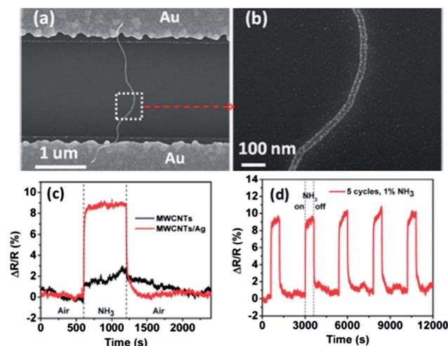
Fig. 1 (a) SEM image of a MWCNT decorated with Ag NCs bridging two gold electrode fingers. (b) Magnified SEM image of the Ag-MWCNT structure as marked in (a). (c) The dynamic sensing response ( $\Delta R/R$ ) of the MWCNT to 1% NH<sub>3</sub> before and after Ag NCs decoration. (d) Five sensing cycles of the Ag-MWCNT hybrid sensor to 1% NH<sub>3</sub>. Reprinted with permission from ref. 23. Copyright 2012 American Chemical Society.
