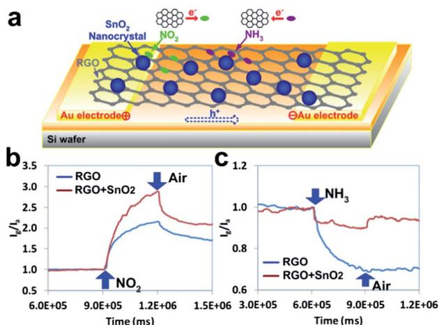
Fig. 3 (a) Schematic of the novel gas-sensing platform of a RGO sheet decorated with SnO<sub>2</sub> NCs. (b) Gas sensing signals of NO<sub>2</sub> and NH<sub>3</sub> from RGO sensors with and without SnO<sub>2</sub> NCs. The sensing signal is normalized by the measured sensor current in air (base line,  $I_g/I_a = 1$ ). Reprinted with permission from ref. 55. Copyright 2012 RSC Publishing.
