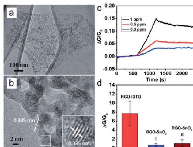
Fig. 4 (a and b) TEM and high-resolution TEM images of RGO–IDTO nano hybrids. (c) Dynamic sensing responses of RGO–IDTO toward different NO<sub>2</sub> concentrations. (d) Sensitivity comparison of RGO–IDTO and RGO–SnO<sub>2</sub> nano hybrids to 100 ppm NO<sub>2</sub>. Reprinted with permission from ref. 68. Copyright 2013 RSC Publishing.
