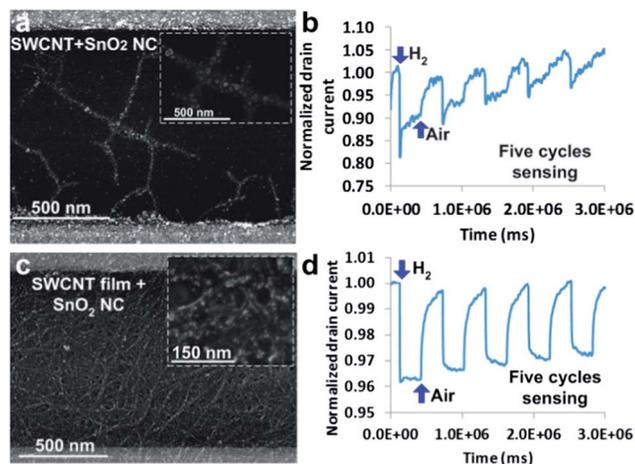
Fig. 2 SEM images of (a) individual SWCNTs and (c) an SWCNT film decorated with SnO<sub>2</sub> NCs. Insets show the magnified images of the hybrid SWCNT–SnO<sub>2</sub> structures. H<sub>2</sub> sensing signals from (b) the SnO<sub>2</sub>–SWCNT and (d) the SnO<sub>2</sub>–SWCNT film sensor for five cycles of sensing. Reprinted with permission from ref. 30. Copyright 2012 RSC Publishing.
