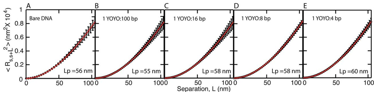
Fig. 4 The mean square end to end distance versus the separation,  $L$  for DNA with (A) no YOYO (B) 1 YOYO per 100 base pairs (C) 1 YOYO per 16 base pairs (D) 1 YOYO per 8 base pairs (E) 1 YOYO per 4 base pairs. The line is the fit to the experimental data using eqn (4). The filled circles are the experimental data obtained by averaging 30 molecules.
