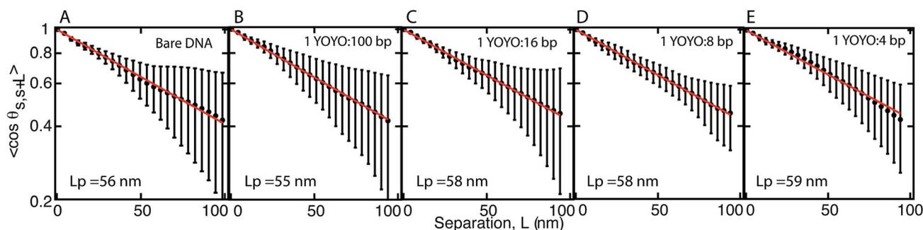
Fig. 3 The correlation function  $\langle \cos \theta_{s,s+L} \rangle$  versus separation,  $L$  for DNA with (A) no YOYO (B) 1 YOYO per 100 base pairs (C) 1 YOYO per 16 base pairs (D) 1 YOYO per 8 base pairs (E) 1 YOYO per 4 base pairs. The filled circles are the experimental data obtained by averaging 30 molecules. The line is the fit to the experimental data using eqn (3).
