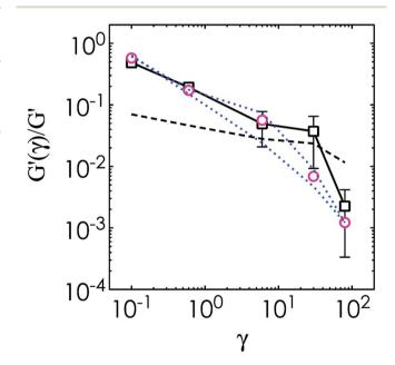
Fig. 4 Comparison of experimental elastic modulus (pink open circles) with high and low frequency bands (blue dotted lines) to theoretical predictions from MCT-PRISM (black dashed line). The modified MCT-PRISM predictions from eqn (3) are shown as open black squares joined by a solid black line. Error bars represent the range of predictions using four different values of the slow MSD (at  $\Delta t = 1.3, 4.5, 9.8$ , and 20.2 s) for each  $\gamma$ .
