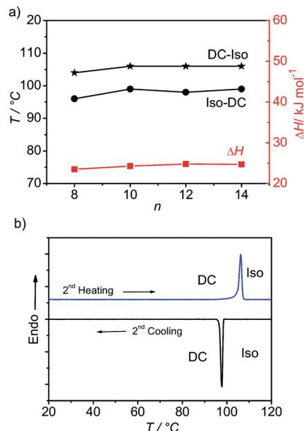
Fig. 2 (a) Dependence of DC–Iso transition temperatures (on heating and cooling scans with  $10\text{ K min}^{-1}$ ) and transition enthalpy values (on cooling from the isotropic liquid) of compounds **BrF8–BrF14** depending on alkyl chain length  $n$  and (b) DSC heating and cooling curves of compound **BrF12** with a rate of  $10\text{ K min}^{-1}$ .
