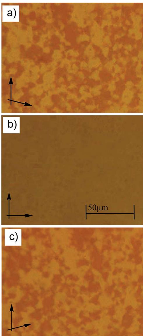
Fig. 1 Textures of the DC phase of compound **BrF12** at  $T = 80\text{ }^{\circ}\text{C}$ : (b) between crossed polarizers and (a) after rotating one polarizer by  $7^{\circ}$  from the crossed position in clock-wise direction and (c) in the anti-clockwise direction, showing dark and bright domains, indicating the presence of areas with opposite chirality sense.
