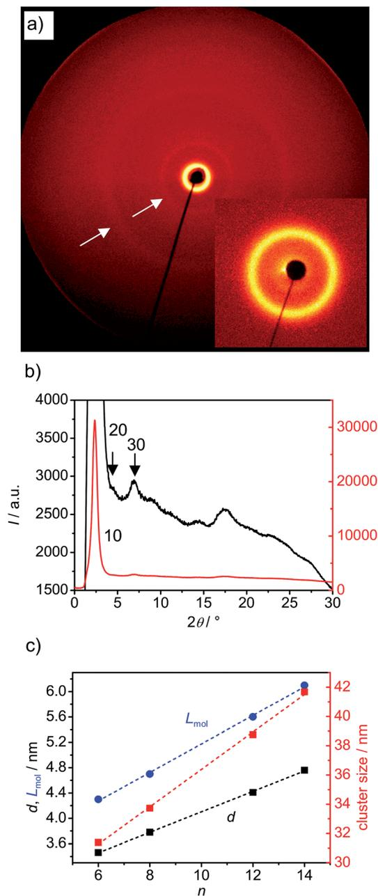
Fig. 3 (a) 2D XRD pattern of the DC phase of **BrF8** at  $T = 90\text{ }^{\circ}\text{C}$ , the inset shows the small angle region; (b)  $2\theta$ -scans over this XRD pattern; (c) dependence of  $d$ -values, molecular lengths ( $L_{\text{mol}}$ ; the used conformation is shown in Fig. S6†) and cluster size (determined using the Scherrer equation and assuming  $K = 1$ ) in the DC phases of compounds **BrF6**–**BrF14** on the chain length.
