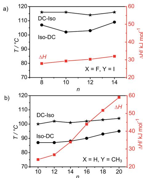
Fig. 6 Dependence of DC–Iso transition temperatures (on heating and cooling scans with  $10 \text{ K min}^{-1}$ ) and transition enthalpy values (on cooling from the isotropic liquid) of two series of compounds related to **BrFn** (a) the 4-iodine-substituted compounds **IF8–IF14** (ref. 43) and (b) the 4-methyl-substituted compounds **M10–M20** (ref. 44) depending on the alkyl chain length  $n$ .
