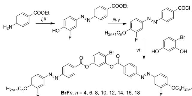
**Scheme 2** Chemical structures and synthesis of compounds **BrF<sub>n</sub>**. *Reagents and conditions:* (i) NaNO<sub>2</sub>, HCl, H<sub>2</sub>O, 0 °C, 30 min; (ii) 1. 2-fluorophenol, NaOH, 0–5 °C, 3 h, 2. NaHCO<sub>3</sub>; (iii) C<sub>n</sub>H<sub>2n+1</sub>Br, K<sub>2</sub>CO<sub>3</sub>, KI, 2-butanone, reflux, 18 h; (iv) 1. KOH, EtOH, reflux, 8 h, (2) H<sup>+</sup>; (v) SOCl<sub>2</sub>, DMF, reflux, 1 h; (vi) TEA, pyridine, CH<sub>2</sub>Cl<sub>2</sub>, reflux, 6 h.
