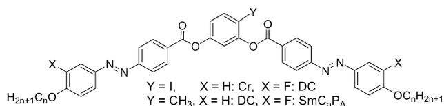
**Scheme 1** Effect of fluorine substitution ( $X = F$  vs.  $H$ ) on the formation of DC phases in azobenzene-based BCLCs (abbreviations; DC = dark conglomerate phase, SmC<sub>a</sub>P<sub>A</sub> = anticlinic tilted antiferroelectric switching SmC phase, Cr = crystalline solid).<sup>43,44</sup>
