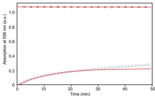
Fig. 5 Absorption at 556 nm as a function of time of the  $\text{Fe}^{2+}$  to  $\text{Ni}^{2+}$  exchange (squares) and of the  $\text{Co}^{2+}$  to  $\text{Fe}^{2+}$  exchange (circles). Lines represent fits of the measured data.
