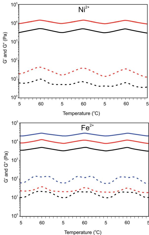
Fig. 8 Temperature dependent storage ( $G'$ , —) and loss ( $G''$ , ---) modulus of  $\text{Ni}^{2+}$  and  $\text{Fe}^{2+}$  8PEG(tpy<sub>5,4</sub>)OH<sub>2,6</sub> ( $\text{M}^{2+}$ -terpyridyl = 1 : 2) hydrogels upon heating to 60 °C and subsequent cooling to 5 °C (three cycles) at different concentrations. Blue, 20 wt%, red, 10 wt% and black, 5 wt%.
