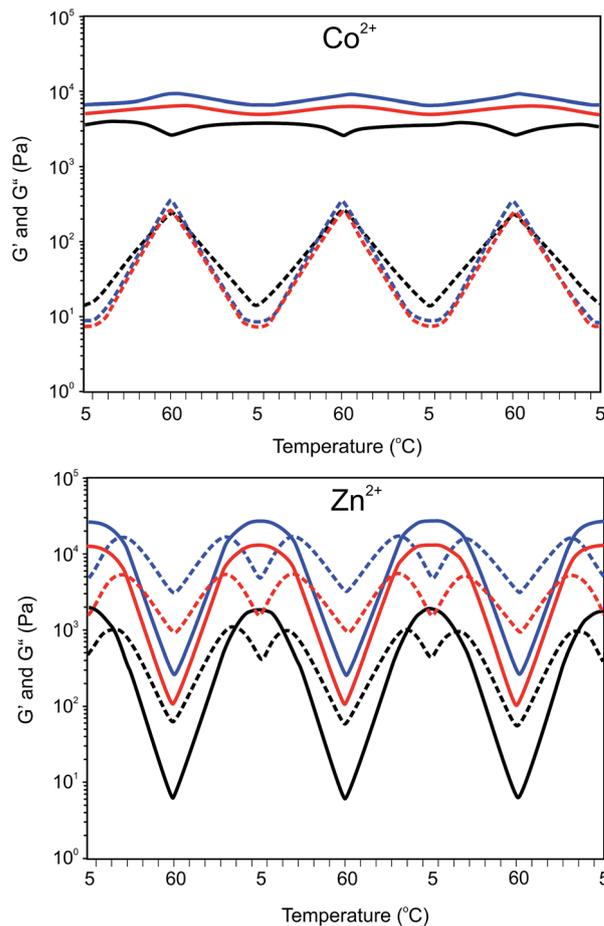
Fig. 9 Temperature dependent storage ( $G'$ , —) and loss ( $G''$ , ---) modulus of a  $\text{Co}^{2+}$  or  $\text{Zn}^{2+}$  8PEG(tpy<sub>5,4</sub>)OH<sub>2,6</sub> ( $\text{M}^{2+}$ -terpyridyl = 1 : 2) hydrogel upon heating to 60 °C and subsequent cooling to 5 °C (three cycles). Blue, 20 wt%, red, 10 wt% and black, 5 wt%.
