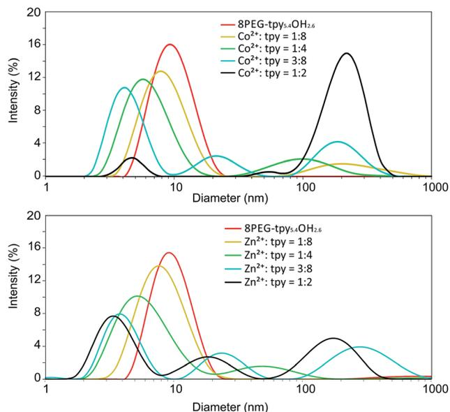
Fig. 7 Nano-particle formation of 8PEG(tpy<sub>5.4</sub>)OH<sub>2.6</sub> with Co<sup>2+</sup> (top) and Zn<sup>2+</sup> (bottom) chlorides at different ratios probed by DLS.
