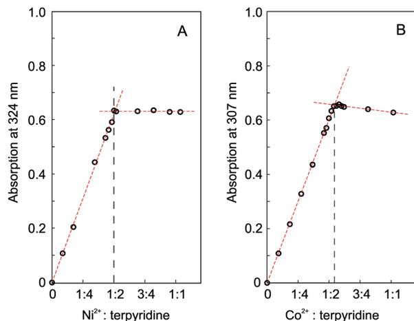
Fig. 3 UV-Vis absorption spectra recorded for the titration of a 8PEG(tpy<sub>5.4</sub>)OH<sub>2.6</sub> solution with a NiCl<sub>2</sub> (A) and CoCl<sub>2</sub> solution (B). Absorption values were determined at 324 nm (Ni<sup>2+</sup>) and at 307 nm (Co<sup>2+</sup>).
