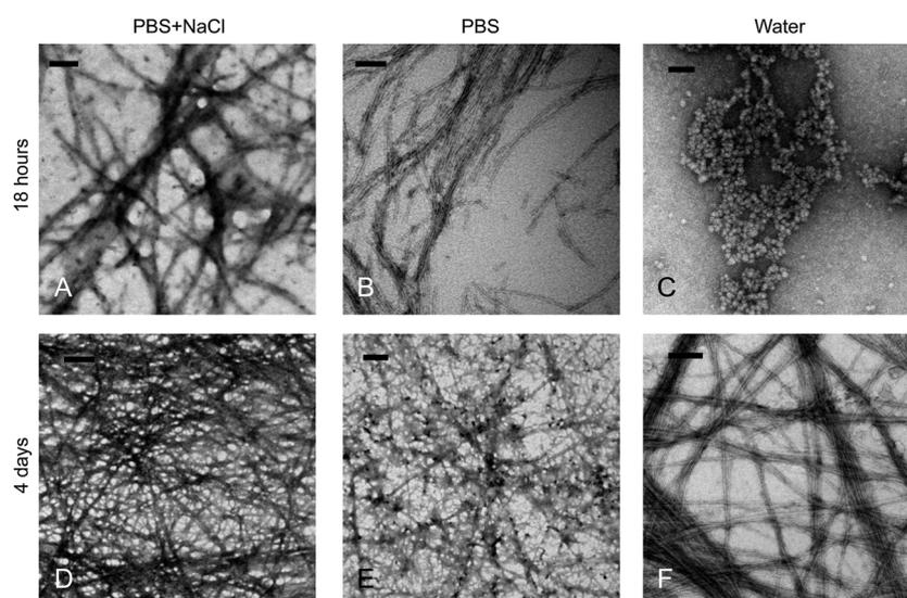
**Fig. 4** TEM images of Fmoc-D-Lac-K-A-8. The depsipeptide was prepared at  $10 \text{ mg ml}^{-1}$  in PBS + NaCl (A and D), PBS (B and E), and water (C and F). The images were collected after 18 hours (A–C, scale bar = 100 nm) and after 4 or 5 days (D–F, scale bar = 200 nm). After 18 hours, relatively short fiber networks are observed in PBS + NaCl and PBS, while globular aggregates are shown in water. After 4 or 5 days, fibers are observed for all samples.
