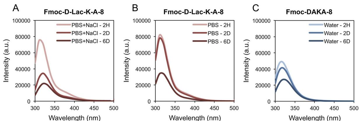
**Fig. 3** Fluorescence emission spectra of Fmoc-D-Lac-K-A-8 in PBS + NaCl (A) and PBS (B) were collected after 2 hours, 2 days, and 6 days. In PBS + NaCl, both a red shift from 310 to 320 nm and decrease in intensity is observed upon the formation of a gel after 2 days. Similarly, the same trend is observed in PBS after 6 days. The peptide equivalent, Fmoc-DAKA-8 forms a gel in water overnight; emission spectra were collected after 2 hours, 2 days, and 6 days in water (C).
