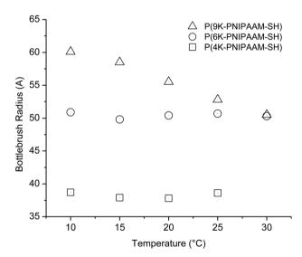
Fig. 5 Bottlebrush polymer radius obtained from Guinier-Porod fitting for 1 wt% PNIPAAM bottlebrush polymers in D<sub>2</sub>O.
