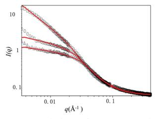
**Fig. 4** Representative SANS data and Guinier–Porod model fits. SANS data for P(9K-PNIPAAM-SH) (square), P(6K-PNIPAAM-SH) (circle), and P(4K-PNIPAAM-SH) (triangle) at 10 °C are shown along with corresponding Guinier–Porod model fits in red.
