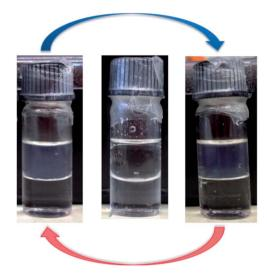
Fig. 8 Micrographs of water/chloroform two-phase mixtures with no polymer added (middle), with 0.1% mass fraction P(6K-PNIPAAM-SH) at room temperature (right), and with 0.1% mass fraction P(6K-PNI-PAAM-SH) at T > LCST (left).
