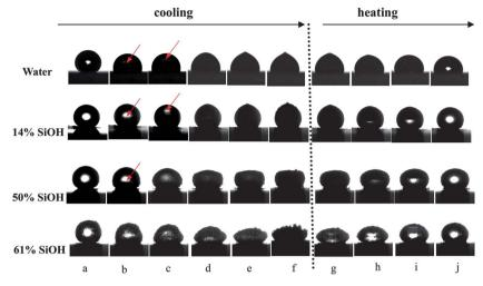
Fig. 2 Shape evolution of a bare water droplet and liquid marbles (15  $\mu$ L) upon freezing (a–f) and re-melting (g–j). The marbles are coated with silica particles of different hydrophobicities (% SiOH). The arrows mark the advancing ice—water interface upwards. The time scales involved in freezing and re-melting are  $\sim$ 90 s.
