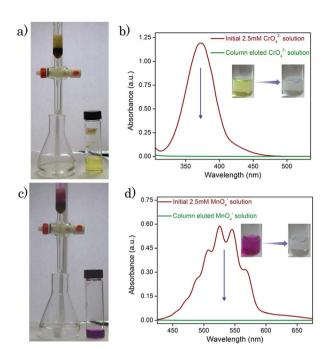
Fig. 3 (a) Image and (b) UV-Vis spectra of the  $2.5 \, \text{mM CrO_4}^{2-}$  solution before and after passing through the compound-1 loaded packed column; (c) image and (d) UV-Vis spectra of the  $2.5 \, \text{mM MnO_4}^-$  ion solution before and after passing through the compound-1 loaded packed column.
