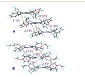
Fig. 3 Single crystal packing diagrams and intermolecular C-H $\cdots$  $\pi$ interactions of (A) TPP and (B) TPP-4M.
