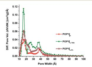
Fig. 4 Pore size distributions based on DFT calculations (slit–pore model) for  $POP1|_a$  (red circles),  $POP1|_{a-TMS}$  (green squares), and  $POP1|_{a-Ph}$  (brown diamonds).
