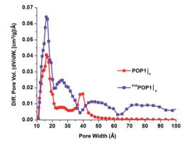
Fig. 5 (Top)  $N_2$  isotherms measured at 77 K of  $POP1|_a$  (red circles) and supercritical  $CO_2$ -processed POP-A (scp $POP1|_a$  — purple squares). Closed symbols, adsorption; open symbols, desorption. (Bottom) pore size distributions based on DFT calculations (slit—pore model) for  $POP1|_a$  (red circles) and scp $POP1|_a$  (purple squares). See ESI† for the isotherms (Fig. S6) and pore size distributions (Fig. S7) of other supercritical  $CO_2$ -processed POPs.
