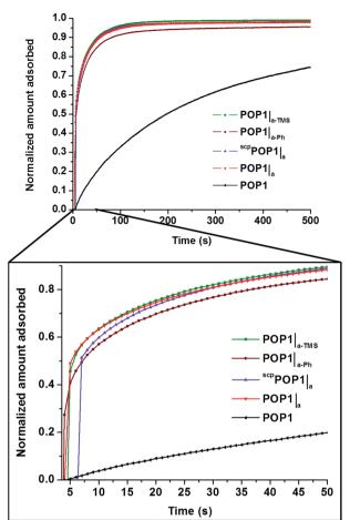
Fig. 6 Time-dependent propane-uptake profiles for POP1,  $POP1|_{a}$ ,  $POP1|_{a}$ ,  $POP1|_{a}$ ,  $POP1|_{a-TMS}$ , and  $POP1|_{a-Ph}$  at 0.3 bar and 298 K. Data in each profile were normalized to the maximum uptake values at 15 000 s (see complete set of data in the ESI,† Fig. S13).
