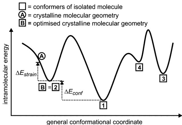
Fig. 1 Schematic of a conformational energy surface, highlighting the conformers of the isolated molecule (1–4), the crystalline geometry (A) and the conformer reached upon energy minimisation of the molecular geometry found in the crystal (B).
