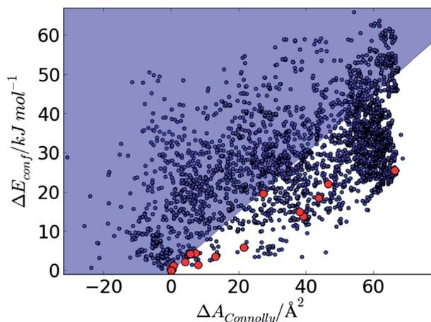
Fig. 7 Plot of  $\Delta E_{\text{conf}}$  against relative Connolly surface area,  $\Delta A_{\text{Connolly}}$  for all predicted conformers of the 15 molecules. Conformers that are observed in the known crystal structures are highlighted in red. The diagonal line represents the gradient of energy vs. surface area derived from Fig. 6.
