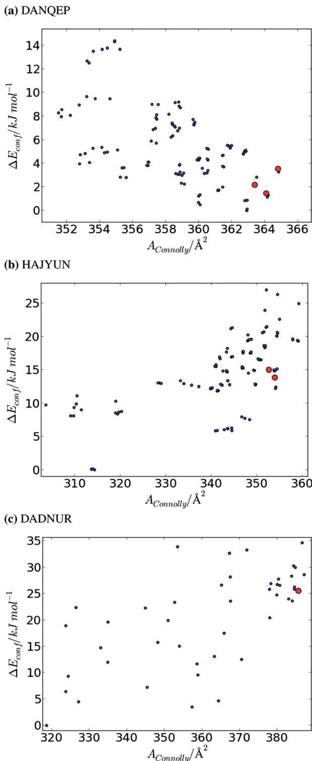
Fig. 5 Plots of  $\Delta E_{\text{conf}}$  against  $A_{\text{Connolly}}$  for all predicted conformers (blue) of (a) DANQEP, (b) HAJYUN and (c) DADNUR. The conformers corresponding to the observed crystal structures are highlighted in red. (a) DANQEP (b) HAJYUN (c) DADNUR.
