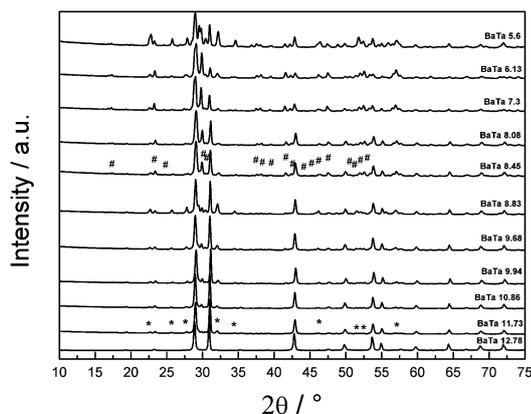
Fig. 1 XRD patterns of prepared barium tantalates *via* citrate route calcined at  $1000^\circ\text{C}$ . The main phase is  $\text{Ba}_5\text{Ta}_4\text{O}_{15}$  with additional phases  $\text{Ba}_3\text{Ta}_5\text{O}_{15}$  (\*) for  $\text{Ba}^{2+}$  amounts of 11.73 mmol and lower added to the synthesis and  $\text{BaTa}_2\text{O}_6$  (#) for  $\text{Ba}^{2+}$  amounts below 8.45 mmol.
