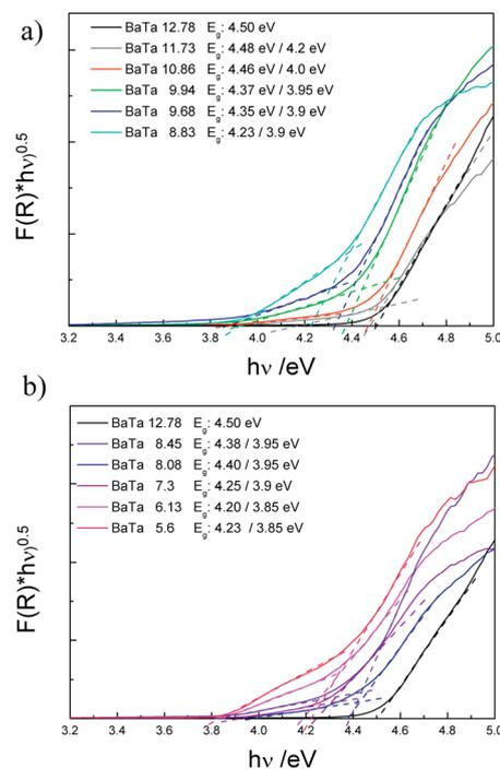
Fig. 2 Tauc plots of  $\text{Ba}_5\text{Ta}_4\text{O}_{15}$  (BaTa 12.78) and its two-component composites (a) and three-component composites (b) *via* diffuse reflectance UV-Vis absorption spectroscopy.
