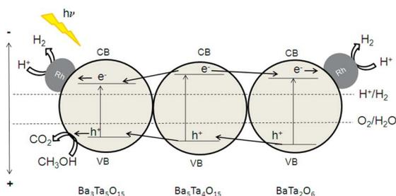
Fig. 8 Calculated band positions of  $\text{Ba}_3\text{Ta}_5\text{O}_{15}$ / $\text{Ba}_5\text{Ta}_4\text{O}_{15}$ / $\text{BaTa}_2\text{O}_6$  (procedure by Butler and Ginley).<sup>38</sup>
