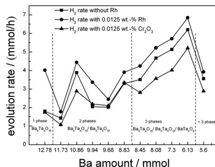
Fig. 7 Screening measurements in  $\text{H}_2\text{O}/\text{MeOH}$  before and after deposition of a specified amount of Rh (0.0125 wt%) as well as step-wise photodeposition of  $\text{Cr}_2\text{O}_3$  on BaTa composites.
