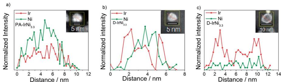
Fig. 5 STEM-EDX line profiles of Ir and Ni in (a) PA-IrNi<sub>3.3</sub> and (b and c) D-IrNi<sub>3.3</sub>. The red arrows in the corresponding NPs (see insets) indicate the directions of the EDX line profiles.
