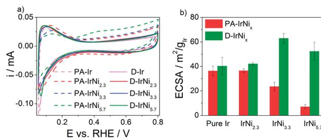
Fig. 4 (a) Voltammetric profiles of the precursor alloy PA-IrNi<sub>x</sub> NPs (dashed) and dealloyed D-IrNi<sub>x</sub> NPs (solid) in N<sub>2</sub>-saturated 0.05 M H<sub>2</sub>SO<sub>4</sub> aqueous solution at 20 mV s<sup>-1</sup>. (b) Comparison of the electrochemically active surface areas of PA-IrNi<sub>x</sub> and D-IrNi<sub>x</sub> NPs.
