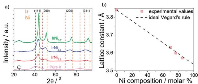
Fig. 2 (a) Powder X-ray diffraction patterns of Ir, IrNi<sub>2.3</sub>, IrNi<sub>3.3</sub>, IrNi<sub>5.7</sub> precursor alloy catalysts; C denotes a support reflection; vertical dashed lines indicate database reflections of pure Ir and pure Ni. (b) the relationship between lattice constant and Ni composition (red symbols) compared to Vegard's law (dashed line).
