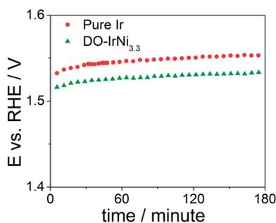
Fig. 9 Chronopotentiometric measurements of pure Ir and directly oxidized (DO) IrNi<sub>3.3</sub> core-shell nanoparticles at a current density of 1 mA cm<sup>-2</sup>.
