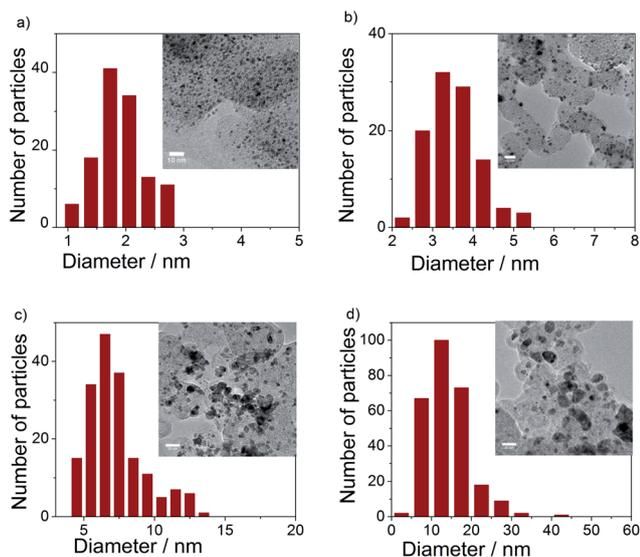
Fig. 3 TEM images and particle size histograms of (a) Ir, (b) IrNi<sub>2.3</sub>, (c) IrNi<sub>3.3</sub>, and (d) IrNi<sub>5.7</sub> precursor alloys.
