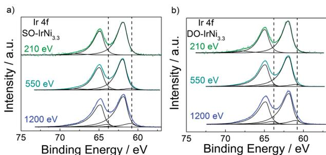
Fig. 7 Ir4f core level spectrum of (a) SO-IrNi<sub>3.3</sub> and (b) DO-IrNi<sub>3.3</sub> at photoelectron kinetic energy of 210, 550 and 1200 eV. Dash lines indicate peak position of metallic Ir as found in PA-IrNi<sub>3.3</sub>.
