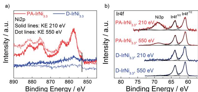
Fig. 6 (a) Ni2p and (b) Ir4f XPS spectra of PA-IrNi<sub>3.3</sub> and D-IrNi<sub>3.3</sub> at photoelectron kinetic energy (KE) of 210 eV and 550 eV. Vertical line in (a) marks the core level shift of metallic Ni.
