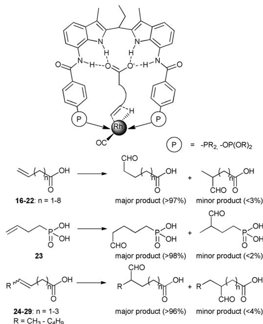
Scheme 6 Binding of substrates to Rh–DIMPhos catalyst in the hydride migration step of hydroformylation (above), and hydroformylation products of substrates **16**–**29** with Rh–DIMPhos catalyst (below).
