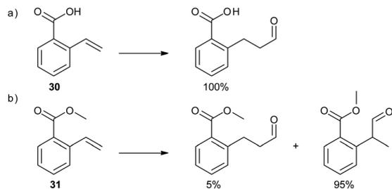
Scheme 7 Influence of substrate preorganization: (a) hydroformylation of substrate **30** that binds to the DIMPhos ligand, and (b) hydroformylation of substrate **31** that cannot bind to the DIMPhos ligand (both with Rh–DIMPhos as catalyst).
