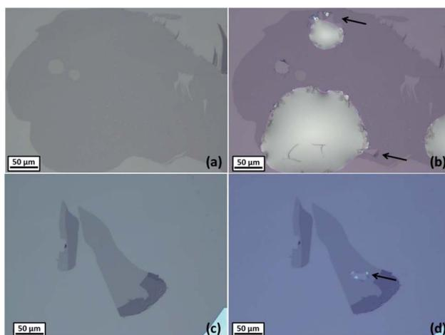
Fig. 4 Optical micrographs of monolayer graphene on Si/SiO<sub>2</sub> before (a) and after (b) the injection of aqueous droplet of 6 M LiCl, and before (c) and after (d) the injection of a droplet of ethylene glycol. Black arrows indicate the holes formed in the monolayer after the droplet deposition.
