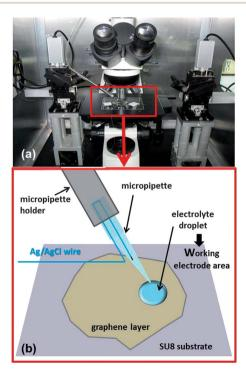
Fig. 1 Photograph of the experimental setup (a). The red rectangle highlights the microscope stage, with the specimen and the micropipette in place. The schematic diagram shows details of the employed two-electrode configuration (b).
