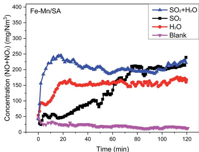
Fig. 1 Catalyst stabilities with catalytic reaction time of 0.12 s at 100 °C under different atmosphere. SO<sub>2</sub>: with 285 mg N<sup>-1</sup> m<sup>-3</sup> SO<sub>2</sub>; H<sub>2</sub>O: with 10 vol% water vapor; SO<sub>2</sub> + H<sub>2</sub>O: with 285 mg N<sup>-1</sup> m<sup>-3</sup> SO<sub>2</sub> and 10 vol% water vapor; blank: without SO<sub>2</sub> and water vapor.
