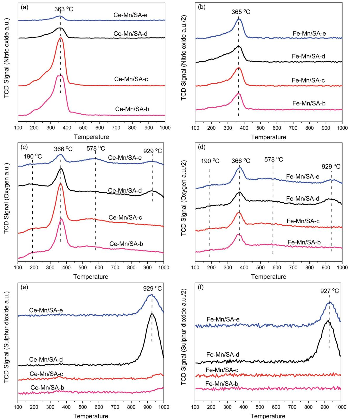
Fig. 5 TPD profiles of NO, O<sub>2</sub>, and SO<sub>2</sub> for catalysts after stability testing. (a) and (b) NO-TPD; (c) and (d) O<sub>2</sub>-TPD; (e) and (f) SO<sub>2</sub>-TPD.
