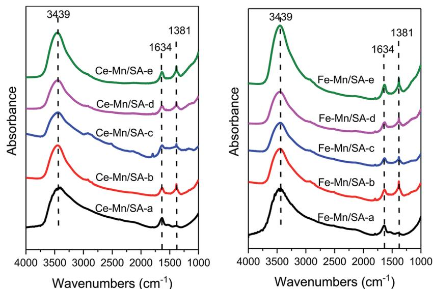
Fig. 7 FTIR profiles of catalysts after stabilities testing.
