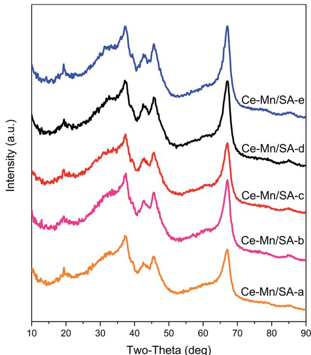
Fig. 2 XRD patterns for Ce-Mn/SA after stability testing.
