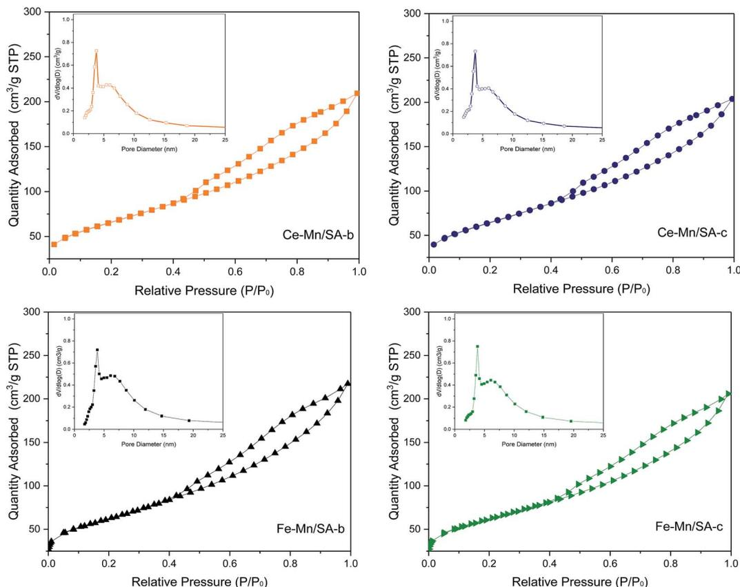
Fig. 3  $N_2$  adsorption–desorption isotherms and pore size distribution curves of Ce–Mn/SA and Fe–Mn/SA after stabilities testing with and without water vapor.
