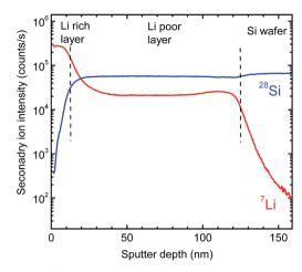
Fig. 3 <sup>7</sup>Li and <sup>28</sup>Si depth profiles as recorded by SIMS.
