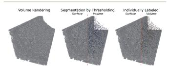
Fig. 8 Volume renderings of the analyzed honeycomb channel aged for 12 h at 950 °C. The segmentation yields all sintered voxels (blue) with high absorption, *i.e.* high Pt concentration, identical to bright regions in the left image. These are further separated into individually labeled blobs, indicated by different colors. Results of the last two steps are presented as view on surface and entire volume.
