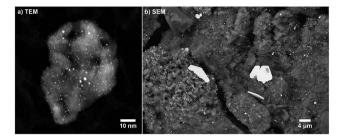
Fig. 3 (a) TEM image (STEM, 910k× magnification) of a fresh Pt/Al<sub>2</sub>O<sub>3</sub> sample. (b) SEM image (BSE, 8k× magnification) of a sample aged for 24 h at 950 °C.
