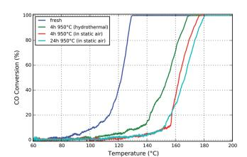
Fig. 1 Light-off curves for CO oxidation for honeycomb samples aged either (i) in static air for 4 and 24 hours, or (ii) with 10 vol%  $\rm H_2O$  in the gas stream for 4 hours.
