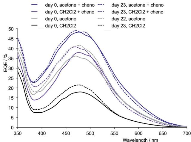
Fig. 2 Dependence of EQE spectra for DSCs with  $[\text{Cu}(1)(4)]^+$  (second-generation with phenyl substituents) on the solvent used in the  $[\text{Cu}(4)_2][\text{PF}_6]$  dye-soaking cycle, and on the use of co-adsorbent cheno.
