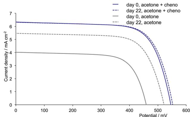
**Fig. 1**  $J$ - $V$  curves for DSCs with [Cu(1)(4)]<sup>+</sup> (acetone used in the [Cu(4)<sub>2</sub>][PF<sub>6</sub>] dipping cycle) on the day of sealing the DSC (day 0) and after 22 days, with (blue curves) and without (grey curves) co-adsorbant cheno.
