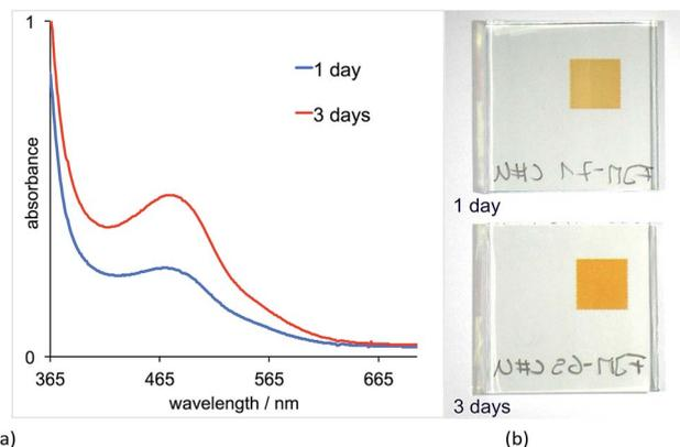
Fig. 4 (a) Solid-state absorption spectra and (b) photographs of electrodes prepared by immersing  $\text{TiO}_2/\text{FTO}$  glass slides (no scattering layer) functionalized with **1** in a  $\text{CH}_2\text{Cl}_2$  solution containing  $[\text{Cu}(\text{MeCN})_4]^+$  and **5** (1 : 1) with dipping times of 1 or 3 days.
