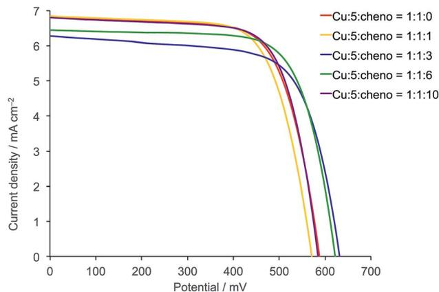
Fig. 5  $J$ - $V$  curves for 7 day old DSCs (see Table 3) in which the dye was assembled by dipping the electrode functionalized with **1** into a dye bath containing  $[\text{Cu}(\text{MeCN})_4][\text{PF}_6]$ , **5** and cheno. The red curve corresponds to a DSC without cheno.
