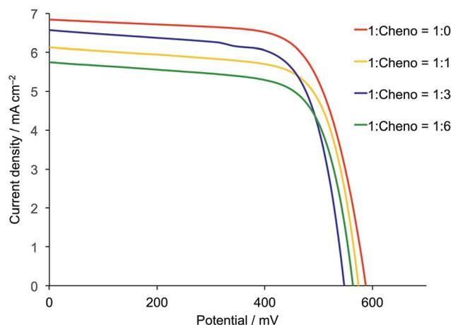
Fig. 6  $J$ - $V$  curves for 7 day old DSCs (see Table 4) in which the dye was assembled by dipping the electrode into a DMSO solution of **1** and cheno (different ratios), followed by treatment with  $[\text{Cu}(\text{MeCN})_4][\text{PF}_6]$  and **5**. The red curve corresponds to a DSC without cheno.
