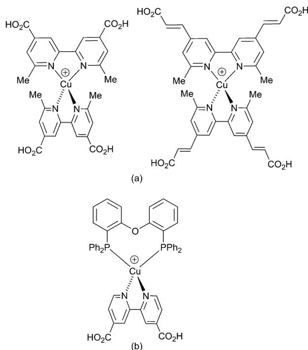
Scheme 3 (a) Two bis(diimine) copper(i) dyes for which the addition of cheno has no effect on DSC performance,<sup>6</sup> and (b) the dye  $[\text{Cu}(4,4'-(\text{HO}_2\text{C})_2\text{bpy})(\text{POP})]^+$  for which addition of cheno results in improved short-circuit current.<sup>23</sup>
