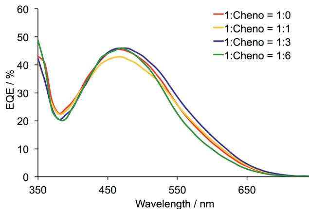
Fig. 7 EQE spectra for 7 day old DSCs in which the dye was assembled by dipping the electrode into a DMSO solution of **1** and cheno (different ratios), followed by treatment with  $[\text{Cu}(\text{MeCN})_4][\text{PF}_6]$  and **5**. The red curve corresponds to a DSC without cheno.
