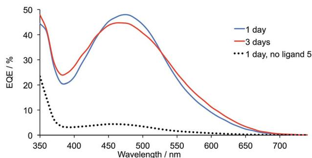
Fig. 3 Comparison of the EQE spectra of 7 day old DSCs with  $[\text{Cu}(1)(5)]^+$  dye assembled by stepwise assembly with a final dipping-cycle of 1 or 3 days (blue and red curves). The dotted line represents the EQE spectrum of a DSC made without addition of ligand 5 to the dye (see text).
