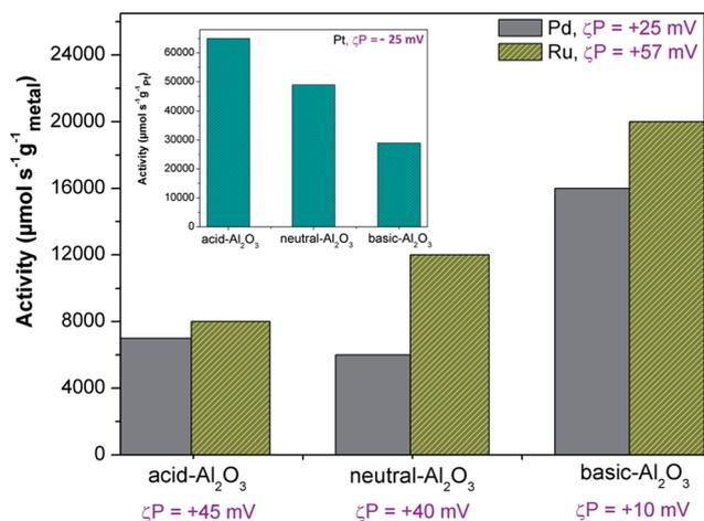
Fig. 7 Activities of Pd and Ru catalysts supported on different acidity of Al<sub>2</sub>O<sub>3</sub> in hydrogenation of methyl crotonate. The inset is activities of Pt catalyst supported on different acidity of Al<sub>2</sub>O<sub>3</sub> in hydrogenation of  $\alpha$ -methyl styrene. The opposite trend of activities between Pt catalyst and Pd and Ru catalysts is because of the different value of zeta potential.
