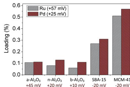
Fig. 5 Loading of supported Ru and Pd catalysts on  $300$  m<sup>2</sup> g<sup>-1</sup> support materials. The amount of metal in the precursor solutions is  $6$  mg.
