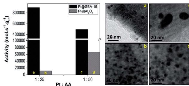
Fig. 6 Activities of the Pt nanodendrites deposited on acidic Al<sub>2</sub>O<sub>3</sub> and SBA-prepared in different molar ratios of Pt to AA and the corresponding TEM images. The larger particles produced by a higher molar ratio of Pt to AA cannot permeate the pores of SBA-15. The lower loadings of Pt@SBA-15 are caused by the same particles charges of Pt and SBA-15.
