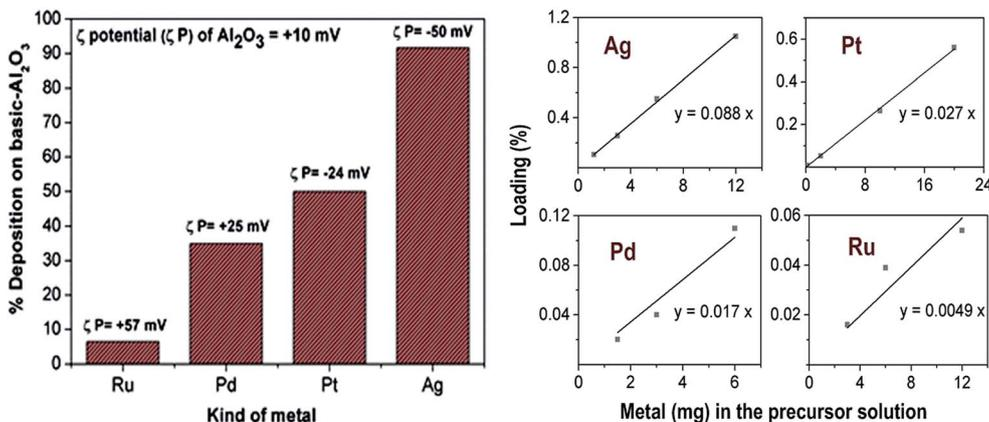
Fig. 4 Left: deposition yields of different metals on basic Al<sub>2</sub>O<sub>3</sub> with a thermo-destabilization method. The amount of metal precursor prepared in each microemulsion system is  $6$  mg. Right: loading of different metal catalysts on basic alumina as a function of the amount (mg) of corresponding metal in the precursor solutions.
