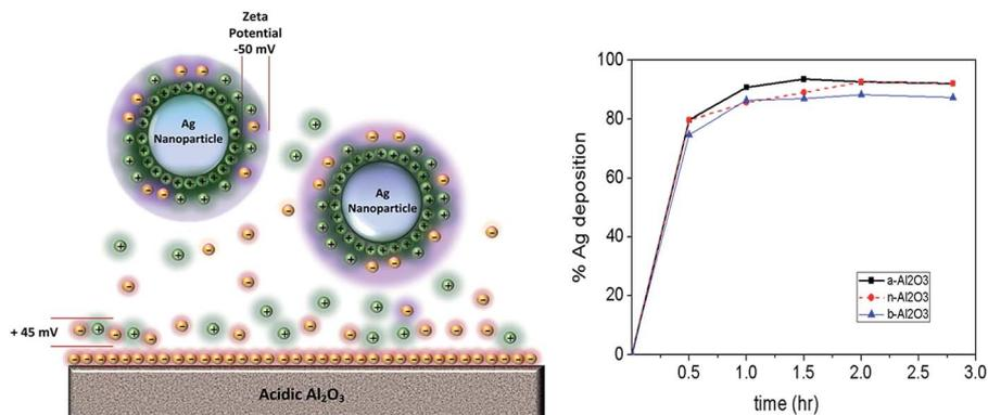
**Fig. 2** Left: schematic illustration of the situation around the support material when Ag NPs are released from the water droplets and then attached onto acidic alumina. Right: deposition yield of Ag NPs on acidic, basic, and neutral alumina based on UV vis spectrometer measurement.
