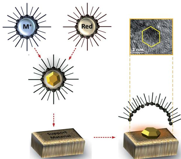
**Fig. 1** Illustration of metal NPs deposition on a support material *via* the thermo-destabilization of microemulsions. The inset is a TEM image of the deposited metal NP. The metal NP which is formed by mixing the one phase microemulsions containing metal precursor ( $M^+$ ) and reduction agent (Red) is deposited onto the support by increasing the temperature above the phase boundary of the microemulsions.
