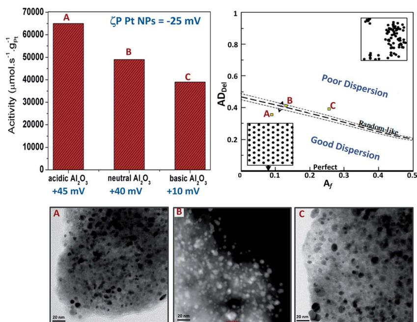
Fig. 8 Upper left: activities of supported Pt catalysts in hydrogenation of  $\alpha$ -methyl styrene. The Pt catalyst was reduced with AA on deposited on acidic (A), neutral (B), basic (C) alumina supports. Upper right: degrees of dispersion of the corresponding catalysts with the Delaunay network method.<sup>34</sup> Bottom: bright and dark field TEM images of the corresponding catalysts.
