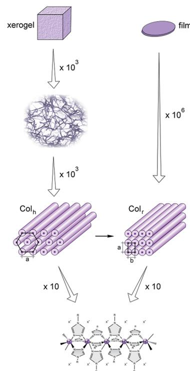
**Fig. 9** Schematic representation of the xerogel and film structures at different scales, showing the columnar hexagonal packing (Col<sub>h</sub>) of the linear stiff rods upon CO<sub>2</sub> critical-point drying, and the columnar rectangular packing (Col<sub>r</sub>) of the linear stiff complexes after solvent evaporation. The Col<sub>h</sub> crystalline structure is a metastable state which transforms towards the more stable Col<sub>r</sub> crystalline structure.
