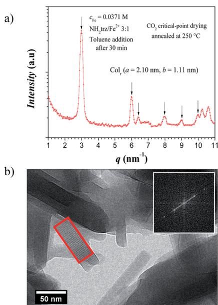
Fig. 6 (a) WAXS 1D scattering profile of the CO<sub>2</sub> critical-point dried gel at  $c_{\text{Fe}} = 0.0371$  M and NH<sub>2</sub>trz/Fe<sup>2+</sup> 3 : 1 annealed at 250 °C showing a columnar rectangular packing of the linear stiff rods. (b) Cryo-TEM image of the annealed CO<sub>2</sub> critical-point drying gel at  $c_{\text{Fe}} = 0.0371$  M and NH<sub>2</sub>trz/Fe<sup>2+</sup> 3 : 1. The inset is the Fast Fourier Transform of the area highlighted in red in the cryo-TEM image.
