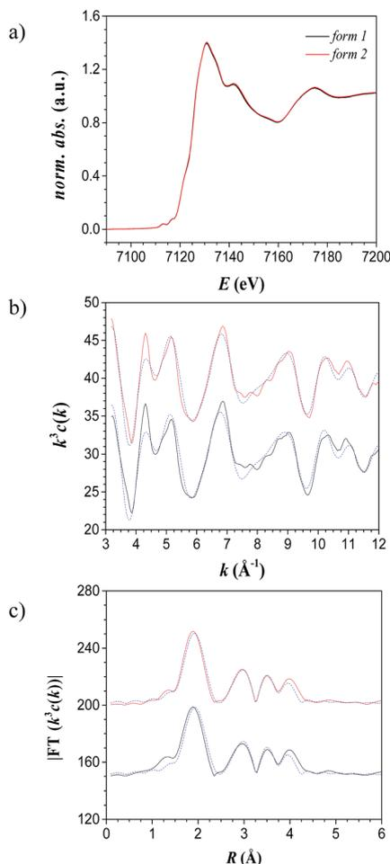
Fig. 1 X-ray absorption spectra of solid  $[\text{Fe}(\text{NH}_2\text{trz})_3](2\text{ns})_2$  as synthesized (black line) and after annealing at  $250^\circ\text{C}$  for 10 min (red line). (a) XANES (b) EXAFS (calculated spectra in blue) and (c) the corresponding Fourier-transformed functions.
