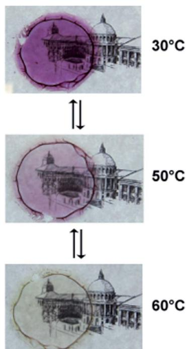
Fig. 7 Photographs of a thermochromic film of [Fe(NH<sub>2</sub>trz)<sub>3</sub>](2ns)<sub>2</sub> prepared from a gel of *type B* at  $c_{\text{Fe}} = 0.0371$  M and NH<sub>2</sub>trz/Fe<sup>2+</sup> 3 : 1 at 30 °C, 50 °C and 60 °C.
