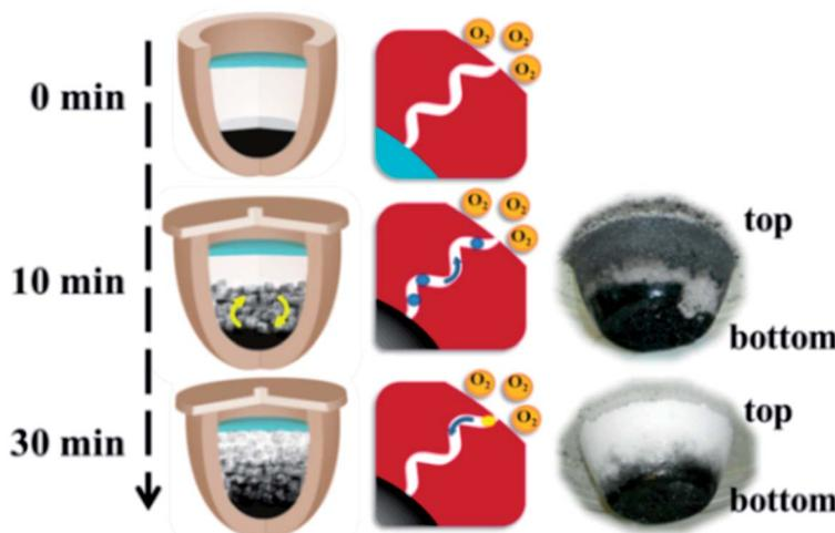
Fig. 4 Illustration of the reaction mixture after 10 and 30 min. The two photographs on the right side show the reaction mixture at 10 and 30 min.
