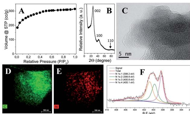
Fig. 2 Characterization of the carbon product  $\text{IL}_1\text{Z}_{0.30}\text{S}_1\text{T}_{30}$ : (A) nitrogen adsorption/desorption isotherm curve; (B) XRD pattern; (C) HRTEM image; (D and E) elemental mapping of carbon and nitrogen elements spectroscopy, respectively (obtained *via* SEM-EDX spectroscopy); (F) XPS spectrum of the nitrogen element.
