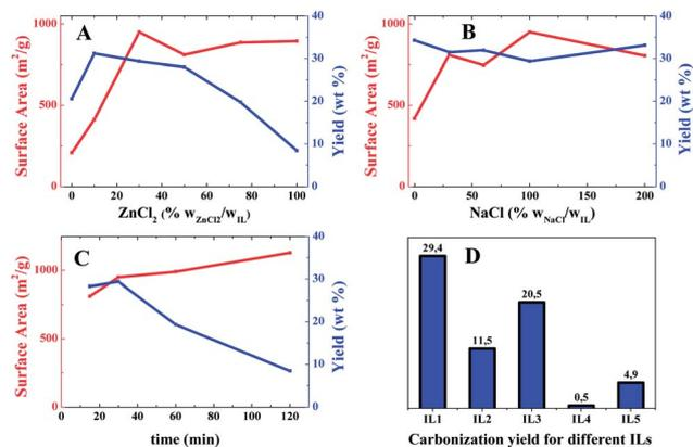
Fig. 3 The variation of the specific surface area and the carbonization yield of the nitrogen-doped porous carbons prepared at different concentrations of  $\text{ZnCl}_2$  (A),  $\text{NaCl}$  (B) and different period (C). Yields from different IL precursors are also reported (D).
