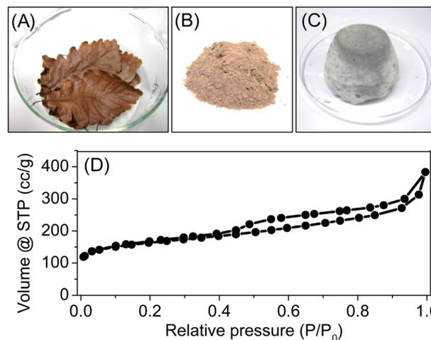
Fig. 5 (A–C) Photographs of pristine oak leaves, grinded powder of oak leaves and sea salt, and the carbonization mixture after 30 min at  $750^\circ\text{C}$ . (D)  $\text{N}_2$  sorption isotherm of the carbon prepared from the oak leaves.
