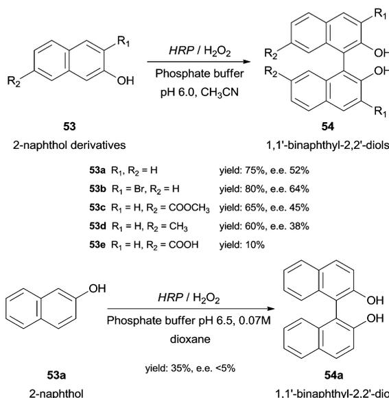
Scheme 16 Biotransformation of 2-naphthol derivatives **53** by HRP.
