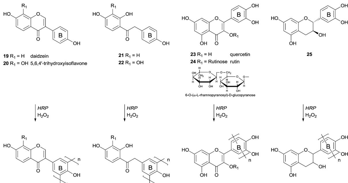
Scheme 8 Polymerization of phenolic compounds by HRP.
