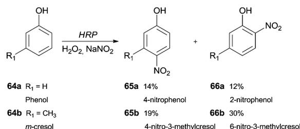
Scheme 20 Nitration reactions performed by HRP/H<sub>2</sub>O<sub>2</sub>/NaNO<sub>2</sub> system with phenol (**64a**) and *m*-cresol (**64b**) as substrates.
