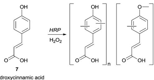
Scheme 2 Chemoselective polymerization of *p*-hydroxycinnamic acid (**7**).
