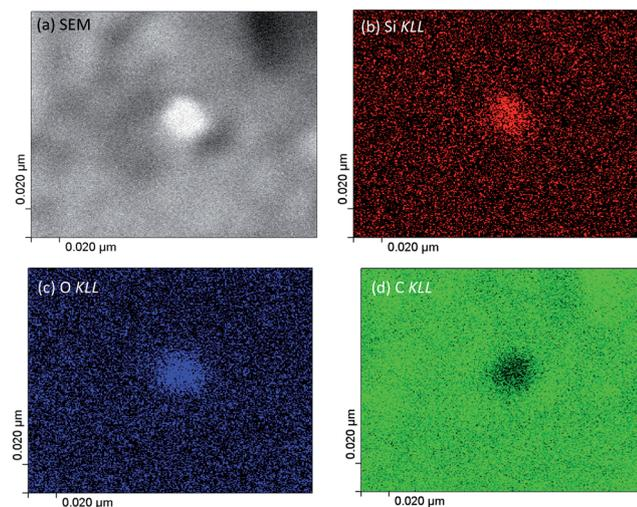
Fig. 7 (a) Image of a silica nanoparticle on a TEM grid taken in the SEM mode of the SAM nano probe applying a 20 keV primary electron beam, (b) Si KLL elemental map, (c) O KLL elemental map and (d) C KLL elemental map.
