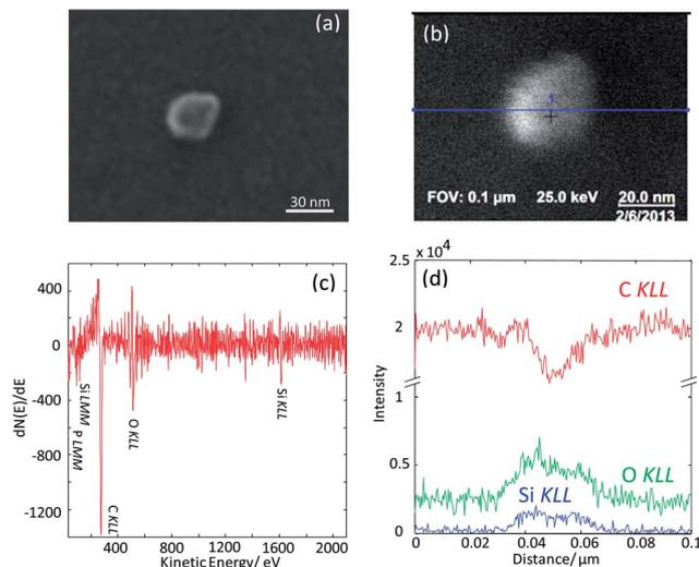
Fig. 6 (a) In-Lens SEM image of a  $\approx 30$  nm silica nanoparticle deposited on a carbon foil of a TEM grid, (b) SEM image of the same particle acquired in the SAM instrument, (c) AES point spectrum taken on the center of the particle identified in (b) and (d) AES line scans across the particle. The line scan position is displayed in (b) with a blue line.
