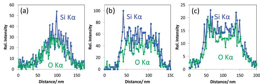
Fig. 4 Representative EDX line scans for Si  $K\alpha$ , obtained on silica nanoparticles (100–150 nm diameter) classified as a) crystalline with the ordered pores therein (class one), (b) amorphous with non-ordered mesopores (class two) and (c) hollow (class three).
