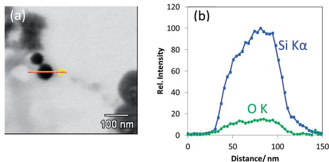
Fig. 5 (a) T-SEM image of a silica nanoparticle ( $d \approx 65$  nm) with an arrow indicating the EDX line scan position and (b) EDX line scan with Si  $K\alpha$  signal and O  $K\alpha$  signal of the particle shown in (a).
