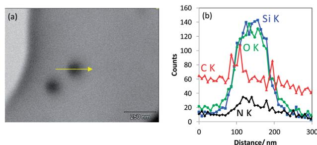
Fig. 9 (a) T-SEM image of non-porous silica nanoparticles covered by an IPTES shell that were deposited on a Substratek™ grid as a low-carbon substrate for analysis, (b) EDX line scan measured along the particle as indicated by the arrow in (a).
