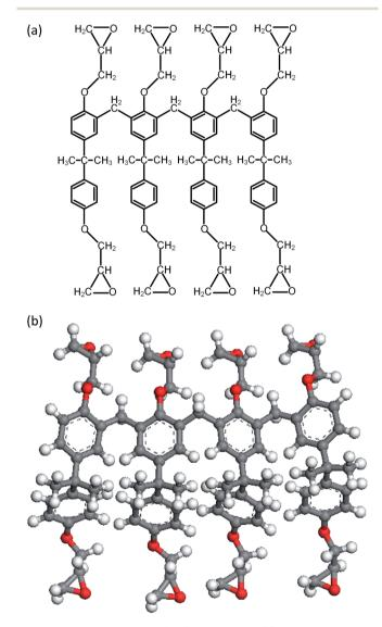
Fig. 1 Epoxy monomer of SU-8 photoresist: (a) chemical structure and (b) molecular model.
