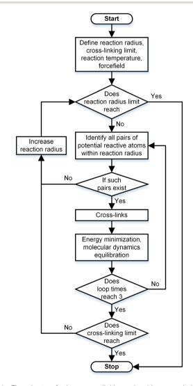
Fig. 2 Flowchart of the cross-linking algorithm used in the construction of epoxy-based materials.
