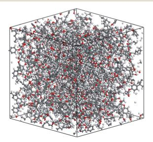
Fig. 4 Cross-linked structure of SU-8 photoresist.
